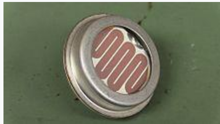
Fig 4.3. Large CdS Photocell from a street light.
