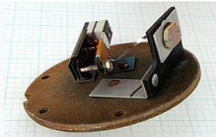
Fig 4.5. The internal components of a photoelectric control
