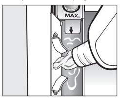
■ Add the fabric conditioner or the liquid starch to compartment ⊗. Do not exceed the maximum level mark
