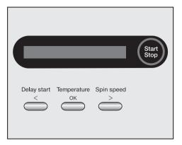
When Further programmes is selected, or in Settings, these buttons have a secondary function. The secondary function is represented by symbols.
