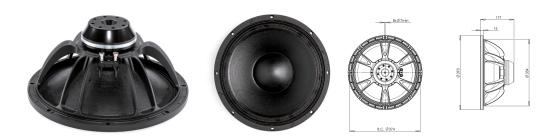
1200 W continuous program power capacity 76 mm (3 in) copper voice coil 40 - 2000 Hz response 100.5 dB sensitivity Aluminium demodulating ring allows a very low distortion figure Neodymium ring magnet assembly
