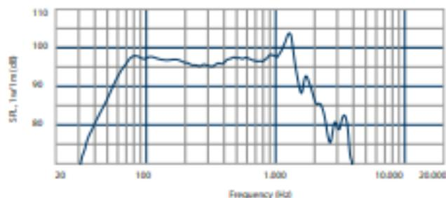
Frequency response curve of the loudspeaker made in a hemispherical, free field and mounted in a reflex box with an internal volume of 55 liters and tuned at 60Hz, applying a sinusoidal signal of 2.83 V @ 8 Ω at 1m.
