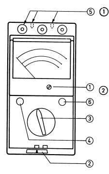
With the current cut off check the zero position adiustment of the pointer. After cleaning the scale window the electrostatic charae should be neutralized by breathing on the glass or touching it or wiping it with a damp cloth.
