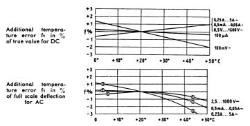
Note: A negative additional error means that the instrument indicates too little; i.e. the true value is obtained by adding the stated percentage to the reading.
