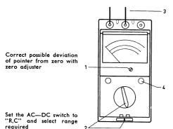
Connect black terminals to AC or DC voltage according to range selected. In capacity measurements the range of the measuring voltage is only valid from 45 to 65 c.p.s. The accuracy is independent of frequency
