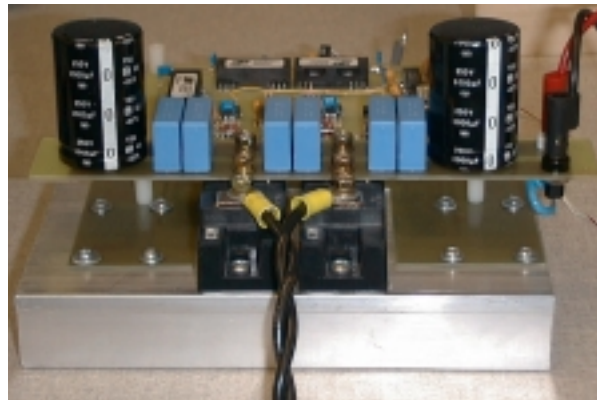
Figure 76: Gate driver inverter hardware
