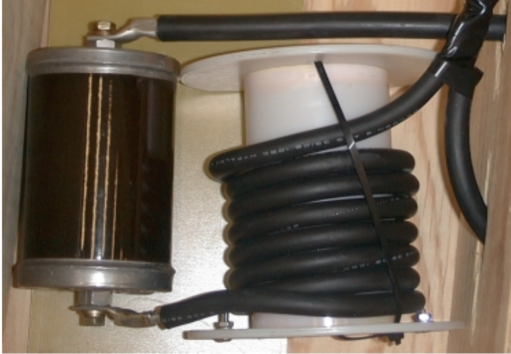
Figure 86: Resonant capacitor and inductor
