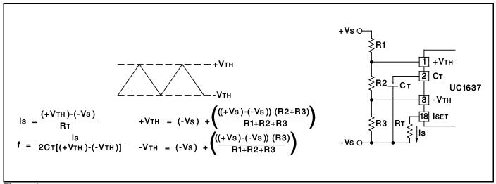
Figure 1. Oscillator Setup
