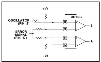
Figure 2. Comparator Biasing
