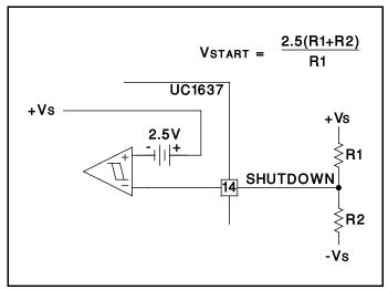
Figure 4. External Under-Voltage Lockout
