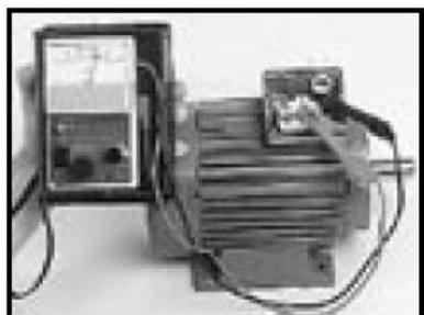
Measuring can be done either on a Y- or D-connected motor. The measuring samples below illustrate 3 different motors A, B and C. The stator winding is measured directly on the motor clutch base. Connect the test cables according to the figures below and compare the phase windings. The measurement values should be almost equal. (A small difference is possible.)
