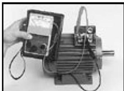
Connect the black test lead to the cover of the object (earth) and the red one to a winding terminal, block terminal or suchlike. Insulation test can be done directly in the starting device, motor plug or suchlike. Push the red button 500 VDC. Read the instrument - red scale graduated in  $M\Omega$ . If the insulation value is low the object should be dismounted, cleaned off, dried or possibly rewinded.
