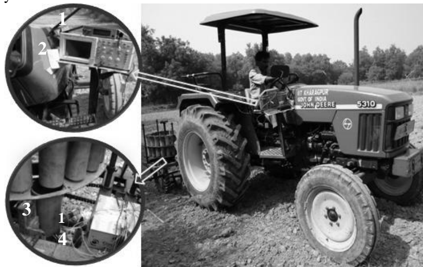
1. Seedling counter 2. Oscilloscope 3. Optoelectric sensor 4. Optical sensor box Fig. 5 Field testing using developed seedling counter
