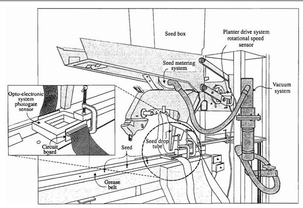
**Figure 1.** John Deere MaxEmerge II planter with the straight metal seed tube (disk openers and press wheel removed) mounted over the grease belt and with the opto-electronic sensor system in place for simultaneous measurement of seed spacing using both systems.
