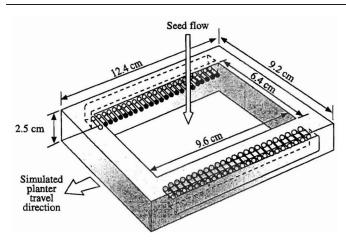
**Figure 2.** Sketch of the opto-electronic system photogate sensor. Twenty-four holes with 3 mm diameter were on each side of the photogate for the LEDs and phototransistors.
