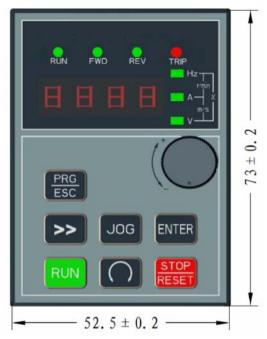
Fig. A5-1 Keyboard Mounting Size of S2R4GB~3004GB
