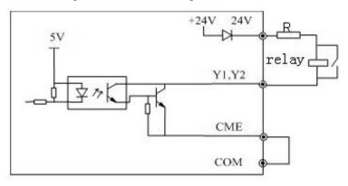
Fig 2-29 Wiring method 1 of multi-function output terminal
