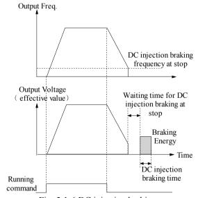
Fig. 5-1-6 DC injection braking
