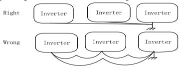
Fig 2-9 Earthling Connection Method
