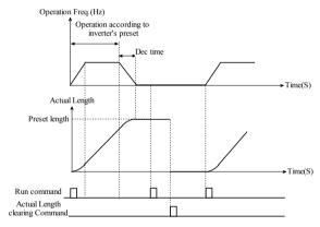
Fig. 5-8-1 Fixed length control diagram
