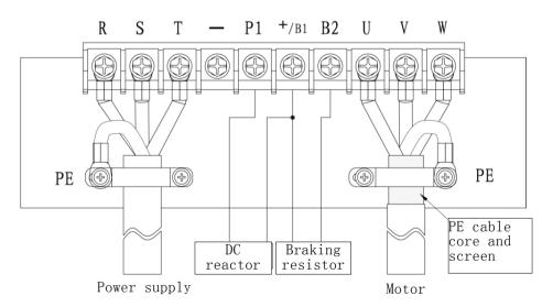
Fig 2-5 35R5GB/37R5PB~3015GB/3018PB Main Circuit Wiring
