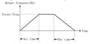
Fig. 5-1-4 Linear acceleration/deceleration
