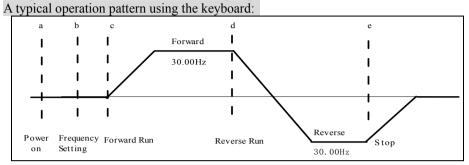
Figure 3-10 Operation sequence by keyboard
