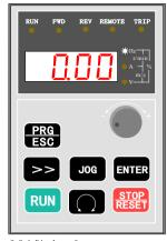
3-3-1 Display of power on. Output frequency is 0.00Hz
