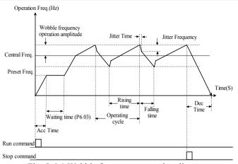
Fig. 5-6-1 Wobble frequency operation diagram
