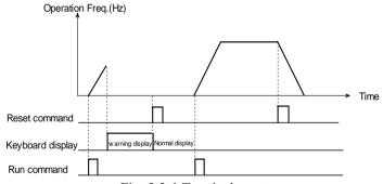
Fig. 5-3-1 Terminal reset
