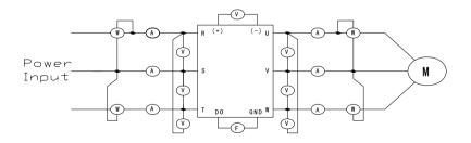
Fig 8-1 Recommendable Wiring of Main Circuit Electro Measurement
