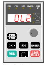
3-3-6 Display of fault state. The fault code is shown and TRIP is on  $\,$
