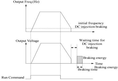
Fig. 5-3-5 DC injection braking
