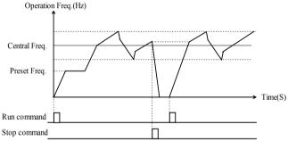
Fig. 5-6-2 Wobble frequency start: continue to operate at the frequency and direction before it stops
