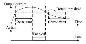
Fig. 5-13-2 Overload pre-alarm function
