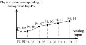
Fig. 5-4-2 Analog input non-linear curve
