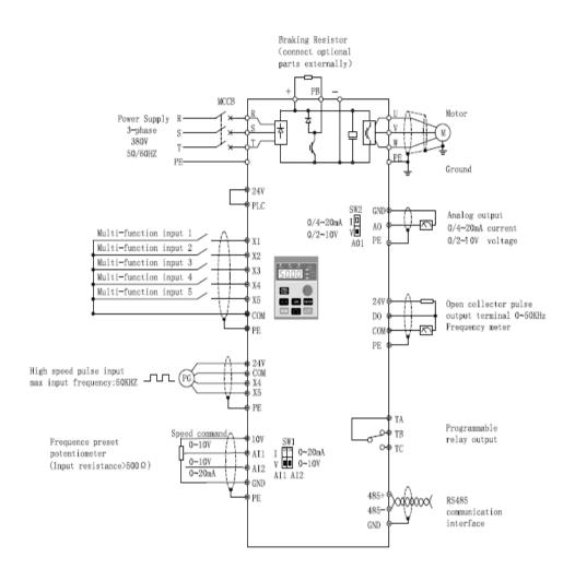
Fig 2-33 3R75GB $\sim$ 3004GB Wiring diagram
