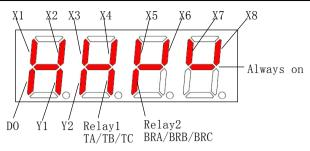
Fig. 5-12-2Terminal status diagram of 35R5GB/37R5PB~3500G
