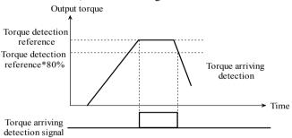
Fig. 5-3-11 Torque arriving detection threshold
