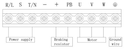
Fig 2-3 S21R5GB $\sim$ S22R2GB Main Circuit Wiring
