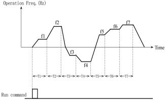
Fig. 5-5-1 Stop mode after single cycle of PLC
