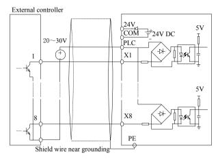
Fig 2-23 Source Connection Method
