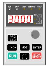
3-3-3 Display of running state RUN is on, FWD blink fast when speed up
