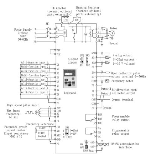
Fig 2-34 35R5GB/37R5PB $\sim$ 3015GB/3018PB Wiring diagram
