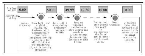
Figure 3-6 Flow chart of frequency setting
