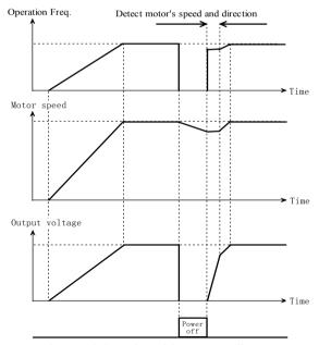
Fig. 5-1-2 Speed tracking restart diagram
