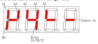
Fig. 5-12-1 Terminal status diagram of S2R4GB $\sim$ 3004GB
