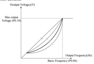
Fig. 5-0-2 Torque-reducing curve
