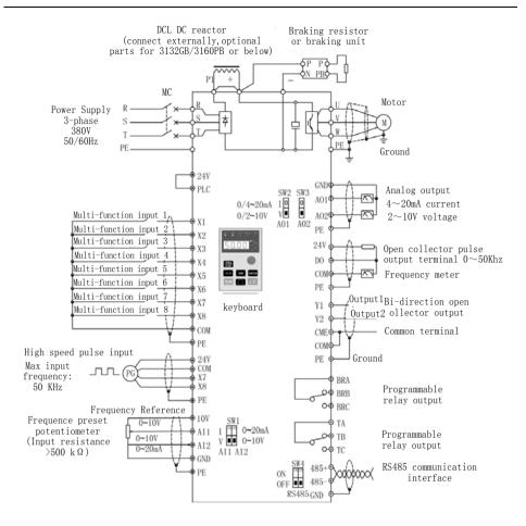
Fig 2-35 3018G/3022P $\sim$ 3500G Wiring diagram
