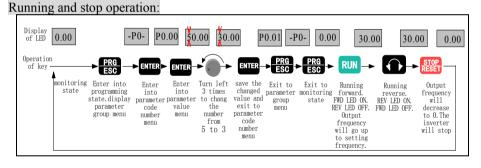
Figure 3-11 Flow chart of running and stop operation
