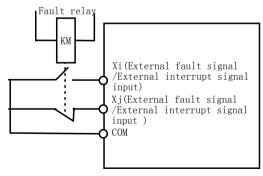
Fig. 5-3-6 Normally open / normally close
