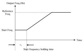
Fig. 5-1-3 Starting frequency and starting time
