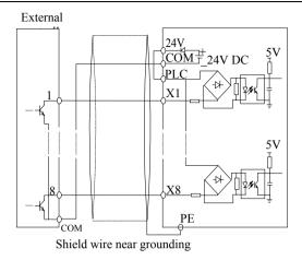
Fig 2-21 Method 2 of connections (a)
