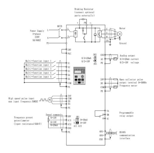
Fig 2-32 S2R4GB $\sim$ S22R2GB Wiring diagram
