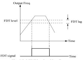
Fig. 5-3-9 FDT level and lag diagram
