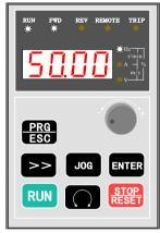
3-3-4 Display of running state RUN is on, the inverter run to the setting frequence and FWD is ON at steady state.
