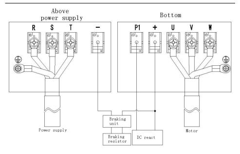
Fig 2-8 3400G~3500G Main Circuit Wiring
