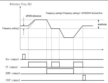
Fig. 5-3-3 UP/DOWN combination operation diagram
