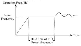
Fig. 5-7-2 PID preset frequency operation
