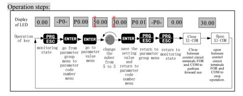
Figure 3-14 Flow chart of running and stop operation by terminal
