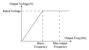
Fig. 5-0-1 V/F characteristic diagram
