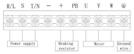
Fig 2-4 3R75GB~3004GB Main Circuit Wiring
