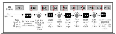
Fig. 5-15-2 Flow chart of user password unlocking
