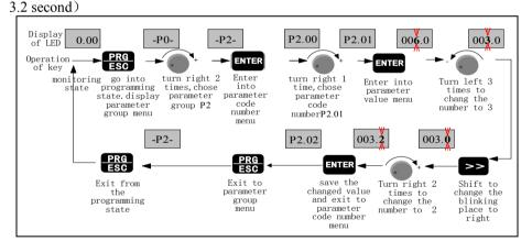
Figure 3-7 Flow chart of parameter setting
