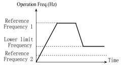
Fig. 5-2-3 Running at Frequency lower limit
