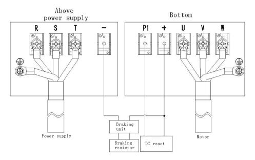
Fig 2-7 3160G/3185P~3355G/3400P Main Circuit Wiring
