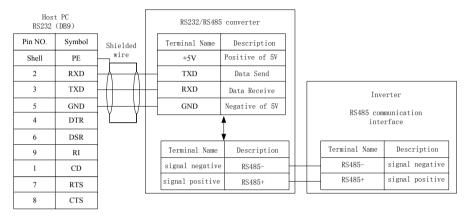
Fig 2-16 Connection between the ac drive and the host PC
