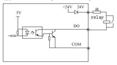
Fig 2-25 Wiring method 1 of DO as switching output
