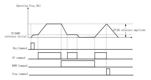
Fig. 5-3-4 UP/DOWN non-combination operation diagram
