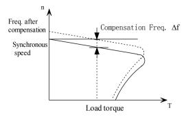
Fig. 5-9-1 Auto slip compensation diagram
