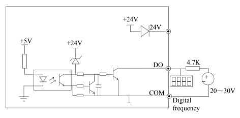
Fig 2-28 Wiring method 2 of DO as pulse output
