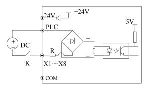
Fig 2-20 Use an external supply
