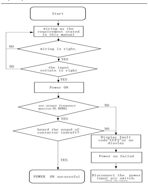
Figure 3-9 Flow chart of the ac drive initialization
