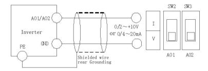
Fig 2-15 35R5GB/37R5PB~3500G Analog output terminal wiring diagram
