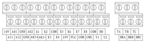
Fig 2-11 S2R4GB~3004GB Arrangement of Control Circuit Terminals
