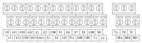
Fig 2-12 35R5GB/37R5PB~3500GB Arrangement of Control Circuit Terminals
