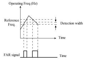
Fig. 5-3-8 FAR detection diagram
