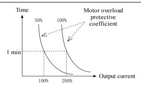
Fig. 5-13-1 Motor overload protection curve
