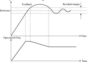
Fig. 5-7-1 Residual margin diagram
