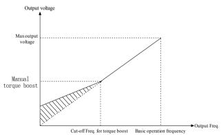
Fig. 5-0-4 Manual torque boost diagram (shadow area is the boost value)
