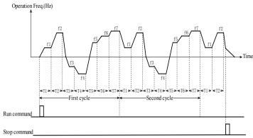
Fig. 5-5-3 Continuous operation of PLC
