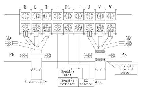
Fig 2-6 3018G/3022P~3055G/3075P Main Circuit Wiring
