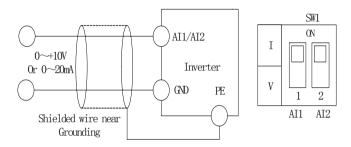
Fig 2-13 Analogy input terminal wiring diagram
