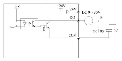
Fig 2-26 Wiring method 2 of DO as switching output
