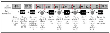
Fig. 5-15-1Flow chart of user password setting
