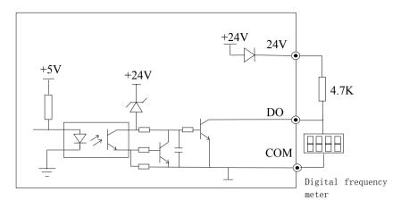
Fig 2-27 Wiring method 1 of DO as pulse output
