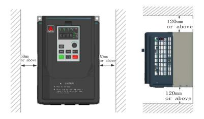
Fig 2-1 Installation Direction and Space
