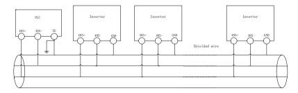
Fig 2-17 Communication between PLC and the Ac drive
