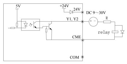
Fig 2-30 Wiring method 2 of multi-function output terminal
