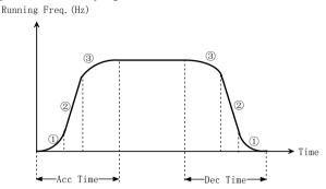
Fig. 5-1-5 S-curve acceleration/deceleration
