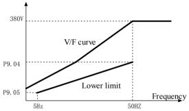
Fig. 5-9-2 Energy saving voltage lower limit
