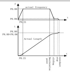
Fig. 5-8-2 Fixed length control diagram 2
