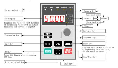
Figure 3-1 Layout and function of Keyboard
