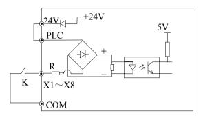
Fig 2-19 Using Internal 24V Power Supply
