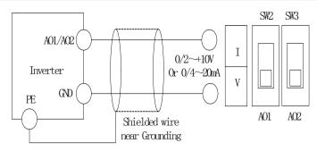
Fig 2-14 S2R4GB~3004GB Analog output terminal wiring diagram
