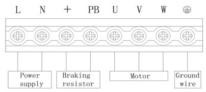
Fig 2-2 S2R4GB~S2R75GB Main Circuit Wiring
