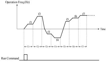
Fig. 5-5-2 Holding the frequency after single cycle
