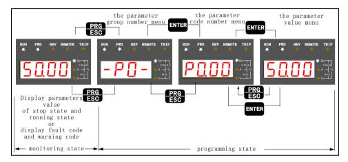
Figure 3-4 Display menus of programming state
