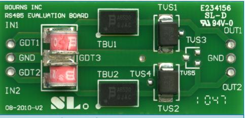
Figure 11: RS-485 Evaluation Board 1: GDT Primary Protector
