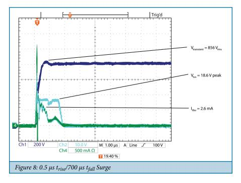
The above power cross and transient surge examples demonstrate the predictable response of the TBU<sup>\*</sup> HSP in limiting current to the protected load. Further, the three-stage protection topology allows the designer to easily select primary and secondary components to provide a robust transient response with minimal verification testing.
