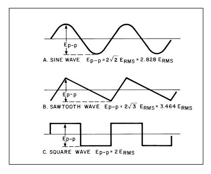
Figure 73. Three Ideal Ripple Waveshapes
