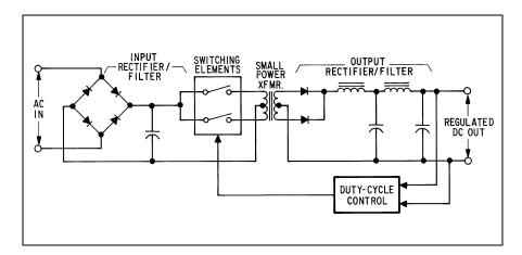
Figure 9. Basic Switching Supply
