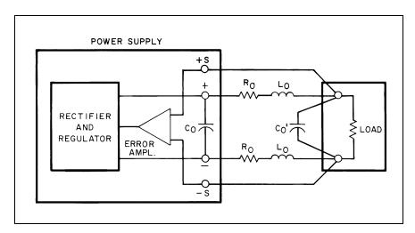
Figure 52. Effect of Load Lead Impedance on Remote Sensing
