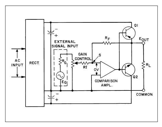
Figure 32. Bipolar Power Supply/Amplifier Drawn as an Amplifier
