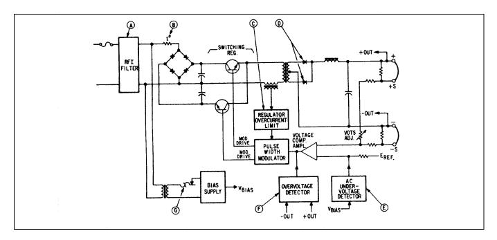
Figure 23. Protection Circuits, Switching Type Supply
