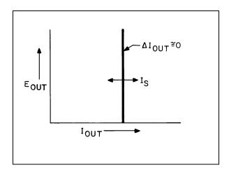
Figure 15. Ideal Constant Current Power Supply Output Characteristic
