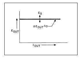
Figure 1. Ideal Constant Voltage Power Supply Output Characteristic
