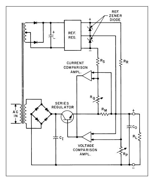
Figure 17. Constant Voltage/Constant Current CV/CC Power Supply
