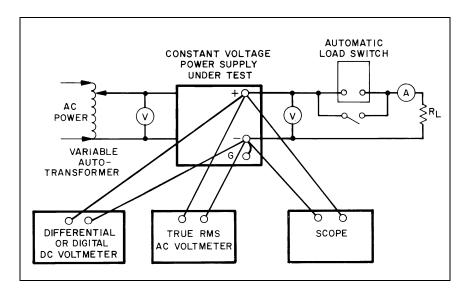
Figure 70. Constant Voltage Measurement Setup
