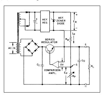
Figure 3. Series Regulated Constant Voltage Power Supply
