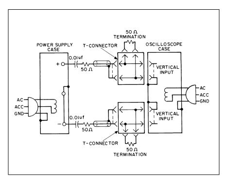
Figure 74. Measurement of Noise Spikes
