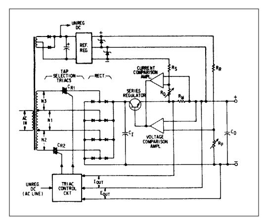
Figure 29. Extended Range Power Supply Using Tap Switching
