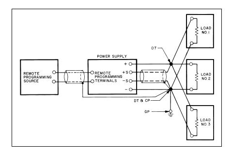
Figure 55. Remote Programming Connections
