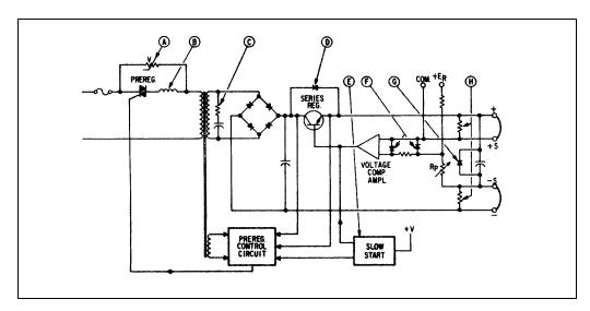
Figure 21. Protection Circuits, Linear Type Supply
