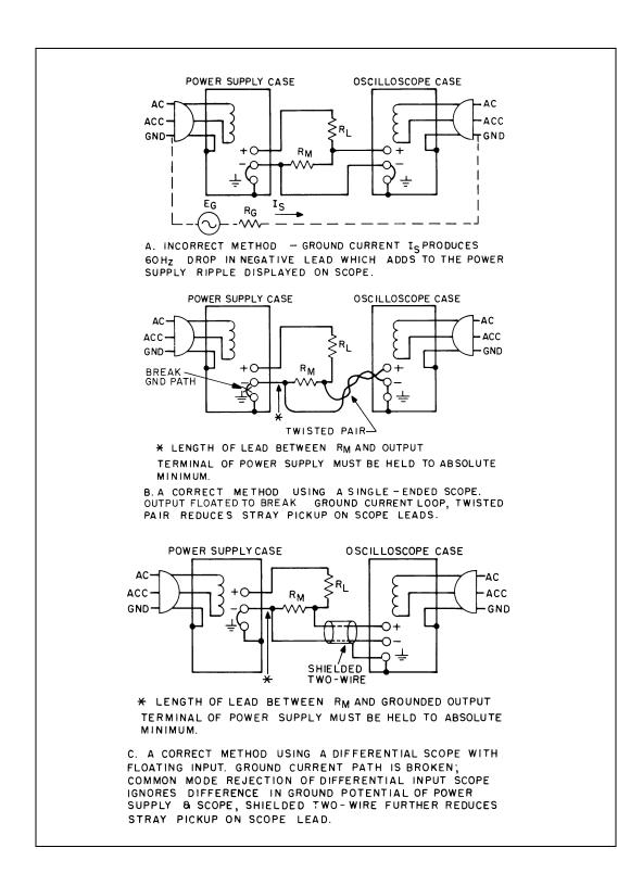
Figure 82. Measurement of PARD for a CC Power Supply
