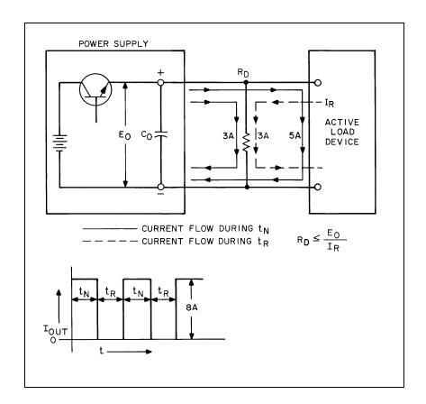
Figure 64B. Reverse Current Loading Solution.
