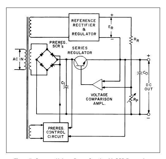
Figure 7. Constant Voltage Power Supply with SCR Preregulator
