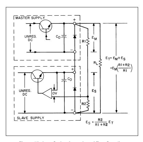
Figure 67. Auto-Series Operation of Two Supplies
