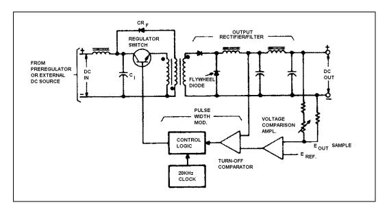
Figure 12. Single Transistor Switching Regulator
