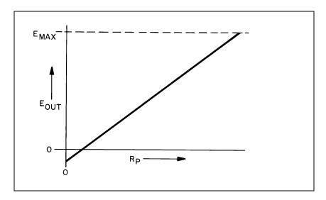
Figure 60. Practical Remote Programming Characteristic
