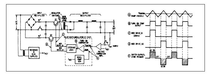
Figure 10. Switching Regulated Constant Voltage Supply
