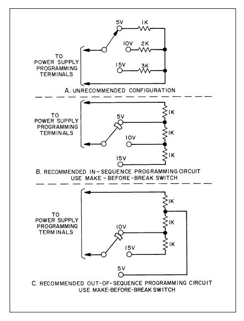
Figure 56. Remote Programming Switching Circuits
