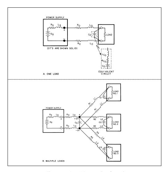
Figure 38. Local Decoupling Capacitors
