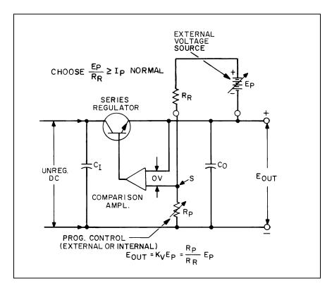
Figure 58. Voltage Programming with Variable Voltage Gain
