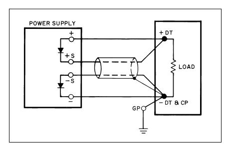
Figure 51. Remote Sensing Protection with Diodes
