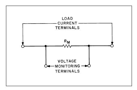
Figure 80. Four-Terminal Current Monitoring Resistor
