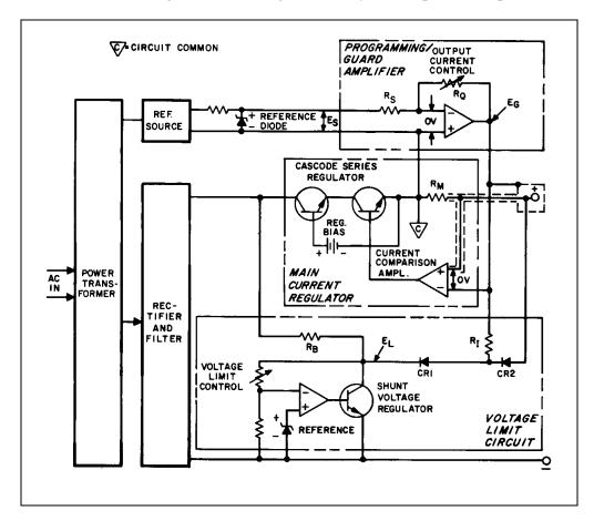
Figure 27. Precision Current Source Block Diagram
