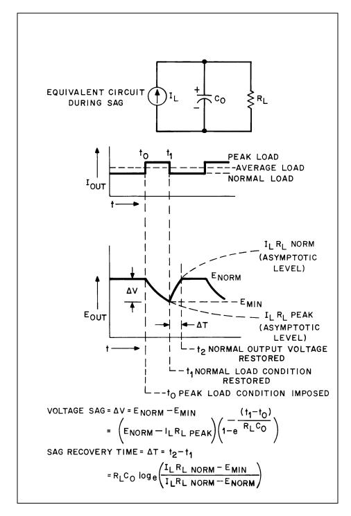
Figure 63. Short-term Overload Equivalent Circuit and Output Voltage
