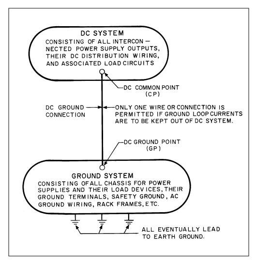
Figure 39. Isolating Ground Loop Paths from DC System
