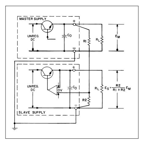
Figure 68. Auto-Tracking of Two Supplies
