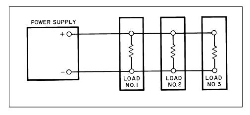
Figure 34. Improper Load Connections
