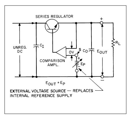
Figure 57. Voltage Programming with Unity Voltage Gain
