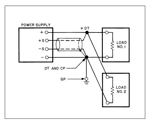
Figure 49. Remote Sensing Connections
