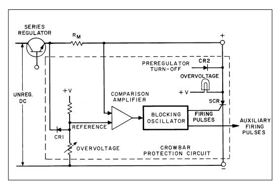
Figure 22. Typical Crowbar Overvoltage Protection Circuit
