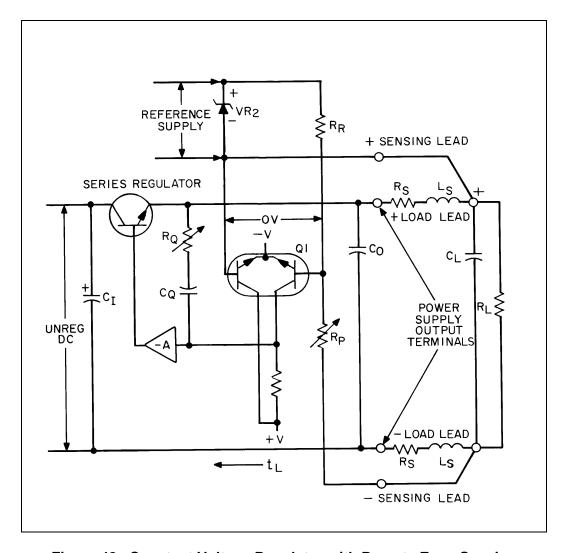
Figure 48. Constant Voltage Regulator with Remote Error Sensing
