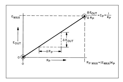
Figure 59. Ideal Remote Programming Characteristics
