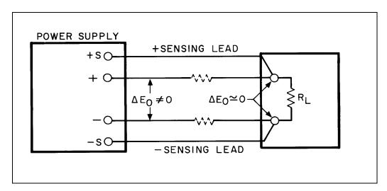
Figure 47. Regulated Power Supply with Remote Error Sensing
