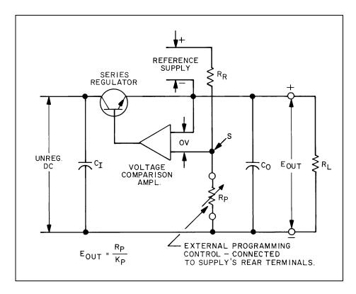
Figure 54. Constant Voltage Supply with Resistance Programming
