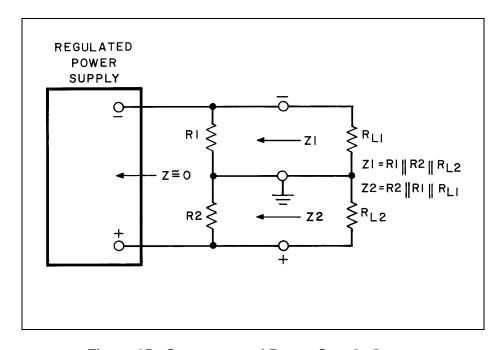
Figure 65. Center-tapped Power Supply Output
