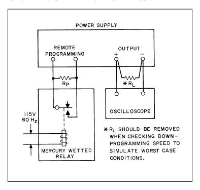
Figure 77. CV Programming Speed Test Setup
