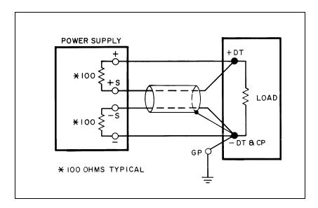
Figure 50. Remote Sensing Protection with Resistors
