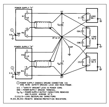
Figure 53. Load Connections for Multiple Power Supplies
