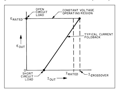
Figure 20. Current Foldback Characteristic
