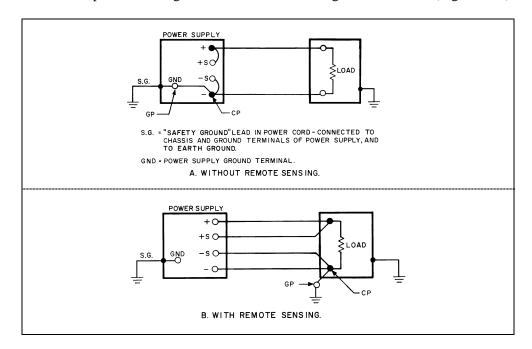
Figure 40. Preferred Ground Connections for Single Isolated Load
