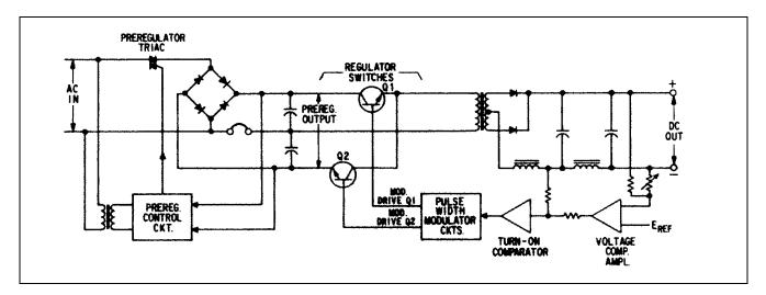
Figure 11. Switching Supply with Preregulator.
