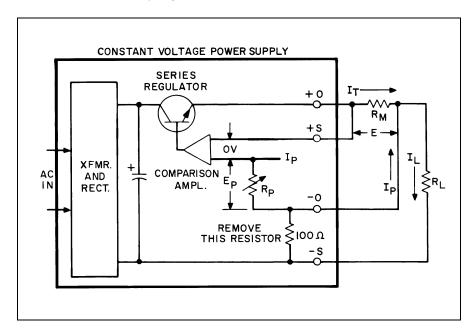
Figure 69. Converting a CV Supply to CC Output
