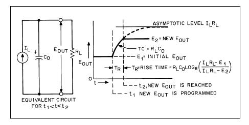
Figure 61. Speed of Response--Programming Up
