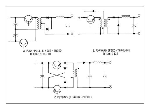
Figure 13. Basic Switching Regulator Configurations
