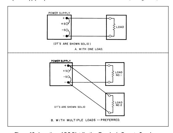
Figure 35. Location of DC Distribution Terminals Remote Sensing
