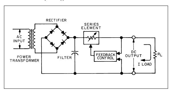
Figure 2. Basic Series Regulated Supply
