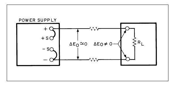
Figure 46. Regulated Power Supply with Local (Normal) Error Sensing
