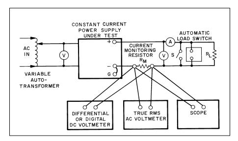
Figure 79. Constant Current Measurement Setup
