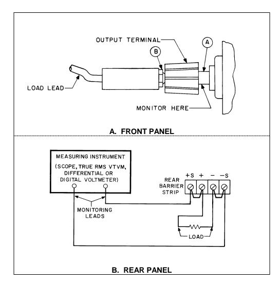
Figure 71. Proper Connections for Monitoring and Load Leads
