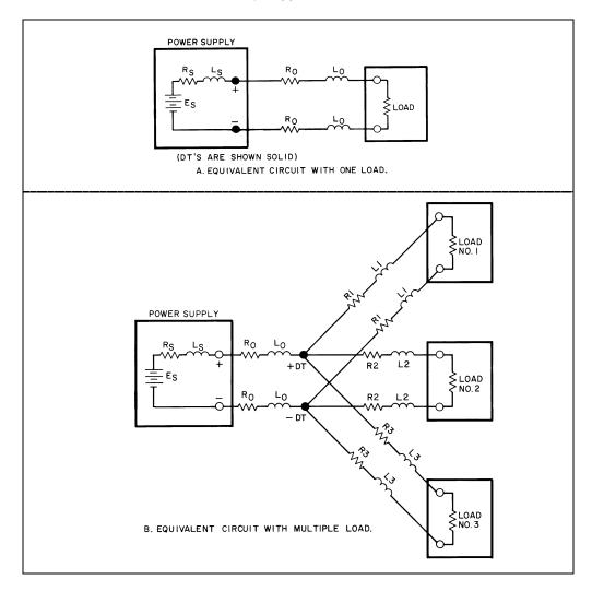
Figure 37. Power Supply and Load Wiring Equivalent Circuits
