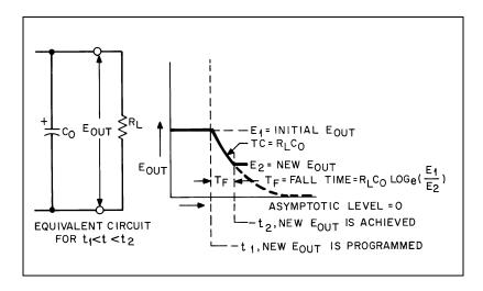
Figure 62. Speed of Response - Programming Down
