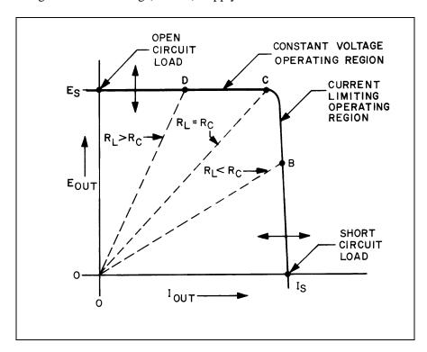
Figure 19. Current Limiting Characteristic
