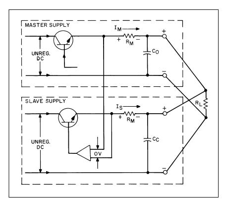
Figure 66. Auto-Parallel Operation of Two Supplies
