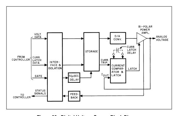
Figure 33. Digital Voltage Source Block Diagram
