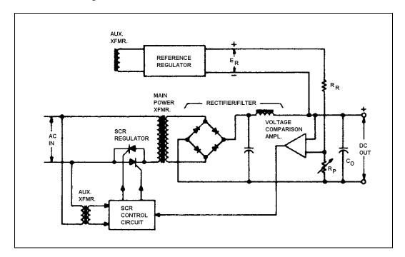
Figure 14. SCR Regulated Power Supply
