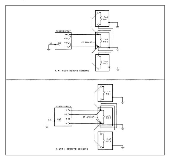
Figure 43. Ground Connections for Multiple Loads, One Grounded
