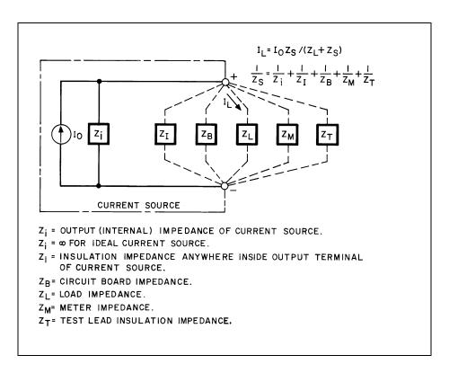
Figure 26. Impedances Shunting the Load Degrade Current Regulation
