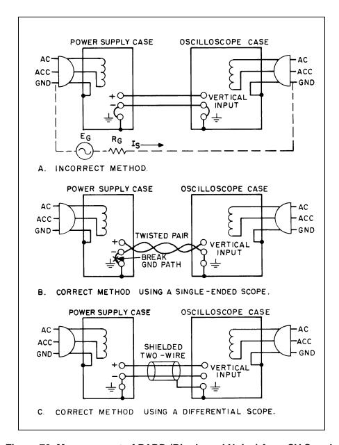
Figure 72. Measurement of PARD (Ripple and Noise) for a CV Supply
