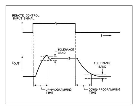
Figure 78. Typical Programming Speed Waveforms
