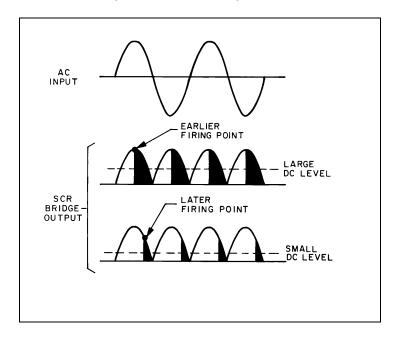
Figure 8. SCR Conduction Angle Control of Preregulator Output
