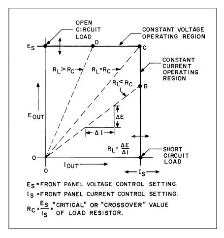
Figure 18. Operating Locus of a CV/CC Power Supply
