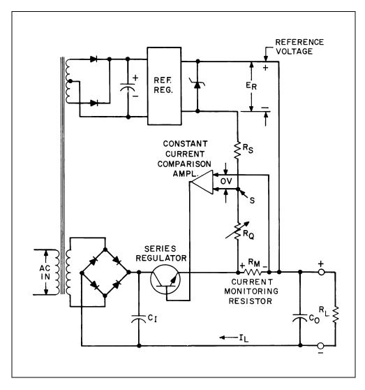
**Figure 16. Constant Current Power Supply**
