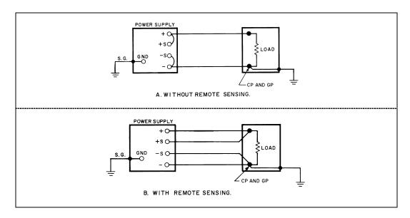
Figure 42. Preferred Ground Connections for Single Grounded Loads
