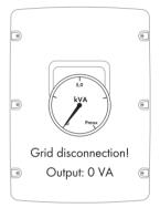
If one of the 3 inverters indicates a device fault and stops feeding in, the other two inverters also disconnect from the power distribution grid 5 minutes later.
