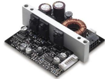
Figure 1: ICEpower250A Size: 8 x 8 x 2.7cm
