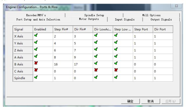
Please note: motor turning direction is relevant to its connection method. If the direction is not right, you can adjust "Dir LowActive" as on the diagram.
