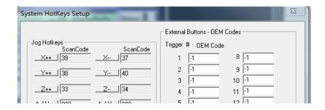
Set the hotkeys of X. Y. Z axis as this diagram, then you can control the motors by this hotkeys on the keyboar.
