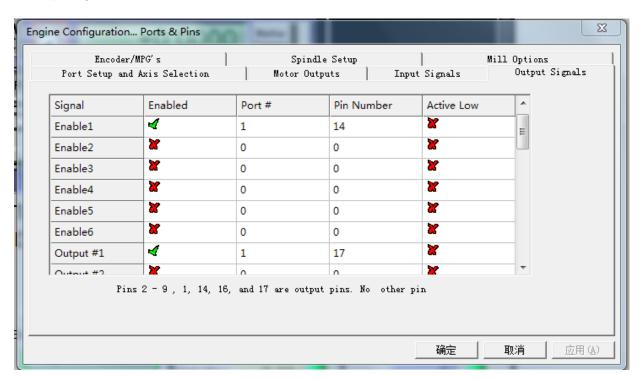
Enable1: stepper motor enable setting. --p14 Output #1: spindle relay switch setting. --P17
