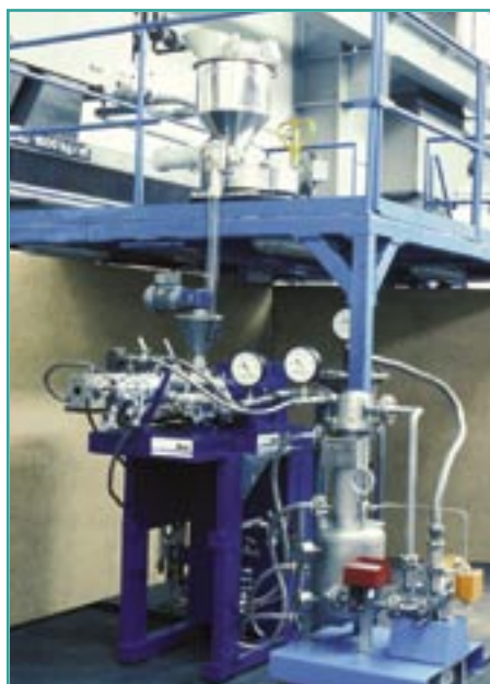
APOVAC-System, Type 136, for the degassing of polymers
