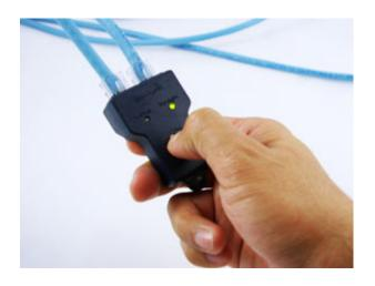
Make sure to test the cables before installing them. An inexpensive Ethernet cable tester does this quite well.
