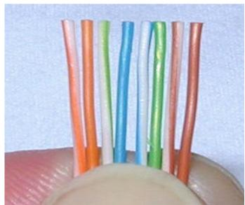
Pinch the wires between your fingers and straighten them out as shown. The color order is important to get correct.
