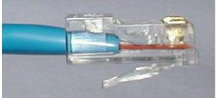
Carefully push all 8 colored wires into the connector. Note the position of the blue plastic sleeve. Also note how the wires go all the way to the end.
