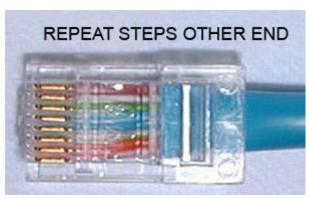
For a standard "Straight Through" cable, repeat all steps and wire color order on the other end of cable. For a crossover cable, the other end will have a different color order as shown by the crossover picture above.
