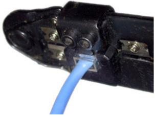
CRIMPING THE CABLE ... carefully place the connector into the Ethernet Crimper and cinch down on the handles tightly. The copper splicing tabs on the connector will pierce into each of the eight wires. There is also a locking tab that holds the blue plastic sleeve in place for a tight compression fit. When you remove the cable from the crimper, that end is ready to use.
