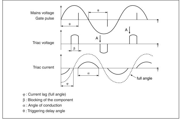
Angle  $\theta$ , characterizing the delay between the mains voltage zero and the triggering pulse, can be adjusted by means of potentiometer P from 0 to 180° to vary the voltage across the load. The current in an inductive load (L.R) lags with respect to the voltage by an angle  $\varphi$ : (tan  $\varphi = L.\omega / R$ ).
