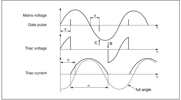
To prevent this fault, it is necessary to insert a "stop" to maintain  $\theta > \phi$ . This is possible for loads whose L and R parameters remain strictly constant.
