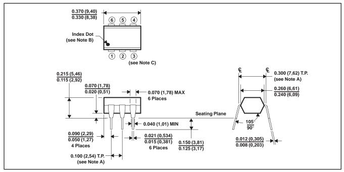
NOTES: A. Terminals are within 0.005 (0,13) radius of true position (T.P.) with maximum material condition and unit installed.
