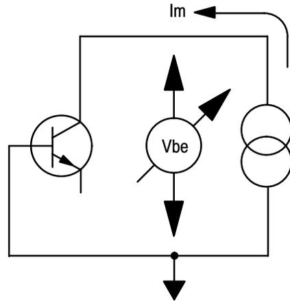
BVCER: reverse Collector to Emitter voltage, the Base connected to the Emitter with a low ohm resistor, under a given Collector current bias.
