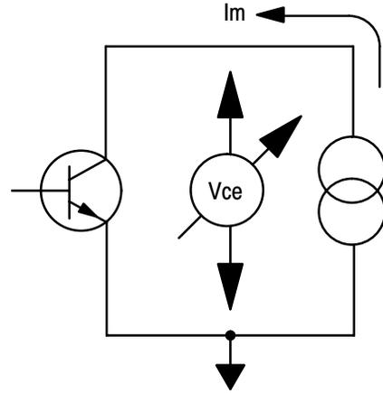
BVCBO: reverse Collector to Base voltage, with the Emitter open, under a given collector current bias.
