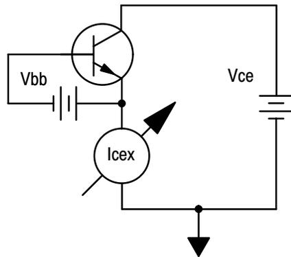
ICEY: Collector to Emitter current under reverse Collector to Emitter voltage, with a forward Base to Emitter bias.
