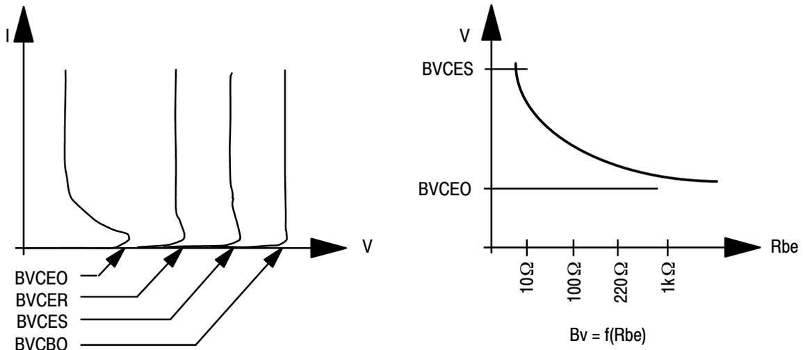
Figure 14. Typical Breakdown Curves (BVEBO not shown)
