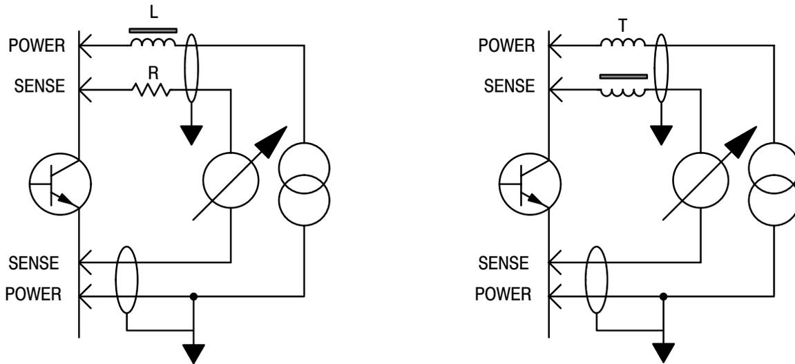
The values of R and L are adjusted for a given transistor and test conditions. Typical values are  $R=470\ \Omega$  and  $L=100\ \mu\text{H}$ . All the network must be located as close as possible to the transistor under test. Kelvin contacts are mandatory. Shielding cables are recommended.
