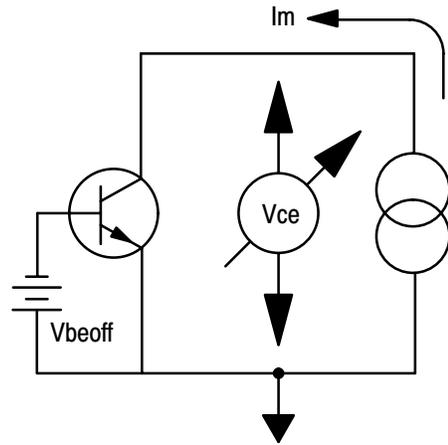
BVCEY: reverse Collector to Emitter voltage, with a forward Base to Emitter bias, under a given Collector current bias.
