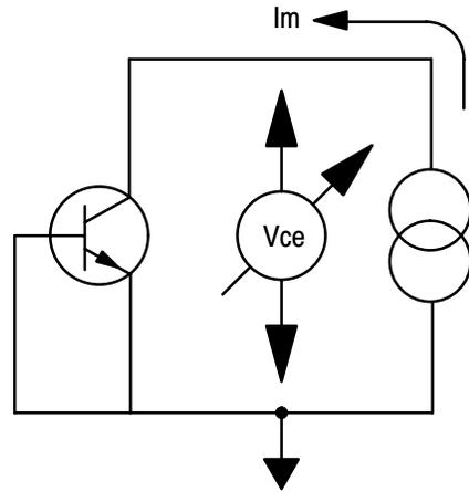
BVCEX: reverse Collector to Emitter voltage, with a reverse Base to Emitter bias, under a given Collector current bias.
