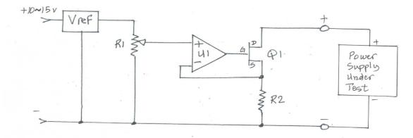
Let's say potentiometer R1 is adjusted so that the voltage on the wiper is 1V. Let's say resistor R2 in the source of the MOSFET Q1 is 1 ohm, and let's say that a 12V power supply is connected between the output terminals (+ on Q1's drain, the upper terminal, and - on the return).
