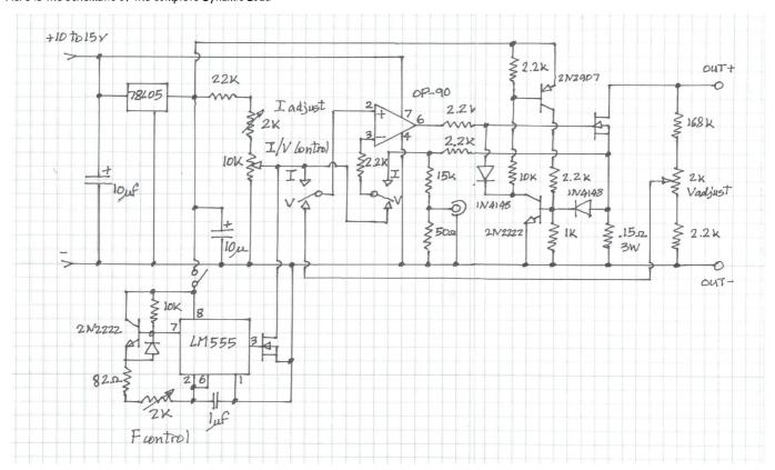
This load can be adjusted for either constant current or constant voltage operation, and includes an oscillator to pulse the load current between 0 and a preselected value at an adjustable rate.
