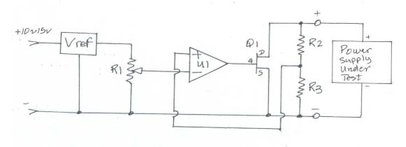
In the Constant Voltage mode, the Dynamic Load does not have current limit, so you must be careful as it is easy to overload a power supply in that mode.
