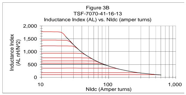
By converting the vertical axis from  $A_L$  value to effective permeability and the horizontal axis from ampere turns (NI<sub>dc</sub>) to magnetizing force (H) the data collected on this core size can be used to predict the capability of any center leg gapped core size and shape (figure 4).<sup>3</sup>
