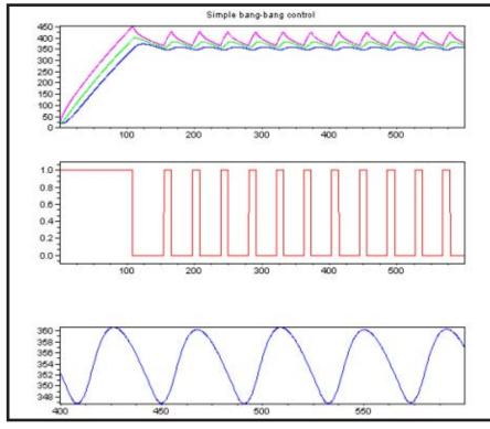
Figure 2-This is the simulation result for a simple "bang bang comparator" system like the one used in the initial version of my iron controller. The top curves are respective heater, tube, and iron temperatures. The middle plot is the power applied on the heater. The bottom curve is a zoom on the tip temperature, showing a 12°C swing around the 350°C target with the parameters I have used.
