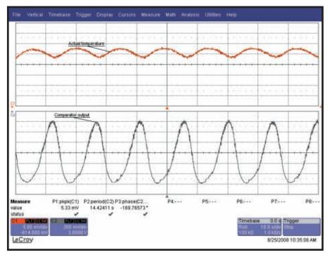
**Photo 3**—This is how the actual iron temperature regulation behaves with the addition of the derivative term. The oscillation of the sensor output is reduced to a little more than 5 mV<sub>pp</sub>, four times less than with the simple comparator, providing a stability of 1°C.
