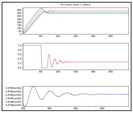
Figure 6—The addition of a derivative parameter gives a PD control loop. Thanks to the derivative, the oscillations are damped out and the system reaches a steady state, at least in this simulation. However, note that the stabilized value is not exactly the preset 350°C. It's a little lower (347.4°C) due to heat dissipation in the ambient air.
