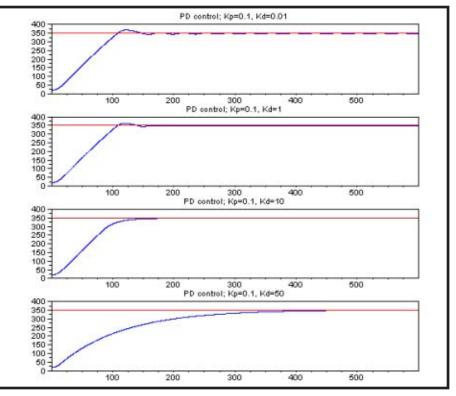
Figure 7—This is what usually happens when the derivative gain Kd is increased. The oscillations are damped more and more. At a given point, the system is no longer oscillating but starts to be long to reach its target. The optimal setting depends on the system constraints.
