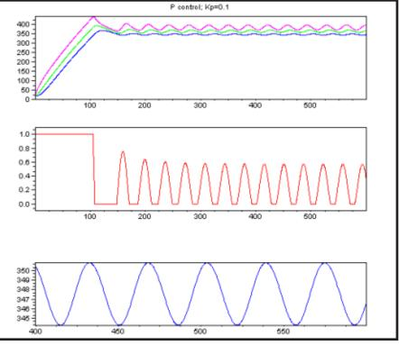
Figure 4—A proportional control enables you to generate an analog output value. It's low if the current measurement is close to the preset target but higher if the target is far (medium curve). The overall temperature oscillation is reduced from 12° down to 7°C, as compared to the "bang-bang" control in Figure 2.
