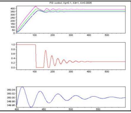
Figure 8—The addition of an integral term enables you to ensure that the steady point is equal to the preset 350°C target. However, note that the oscillations and stabilization time are a little higher than with a simpler PD control loop as on Figure 6.
