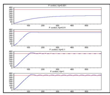
**Figure 5**—This simulation shows you the behavior of the simulated system with a proportional control and different values of the Kp gain. With small Kp values (top plot), the actual temperature takes a long time to reach the target, and may not reach it. The loop is "soft." If you increase the Kp gain, the regulation becomes quicker and quicker up to a point where overshoot starts to appear. The optimum value is often just after the appearance of oscillations (Kp = 0.1 in this instance).
