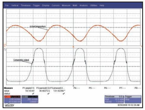
**Photo 2**—This plot was taken on my new LeCroy WaveRunner 6050A oscilloscope connected to the iron controller in its initial version. The top channel is the sensor measurement. The bottom is the command sent to the output TRIAC. In this first design, I used a simple comparator. Both curves are exactly in phase; but as a consequence, the oscillation is high due to thermal inertia:  $19 \text{ mV}_{pp}$  corresponding to 6°C. Heating cycles are roughly 30 s each.
