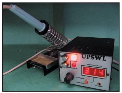
**Photo 1—**This is the power supply and controller I built in 1987 and its Weller VR20 soldering iron. Its first basic "threshold comparator" design was working, but it had a  $\pm 3^{\circ}$ C oscillation around the preset temperature. A simple control improvement reduced the oscillation to  $\pm 1^{\circ}$ C.
