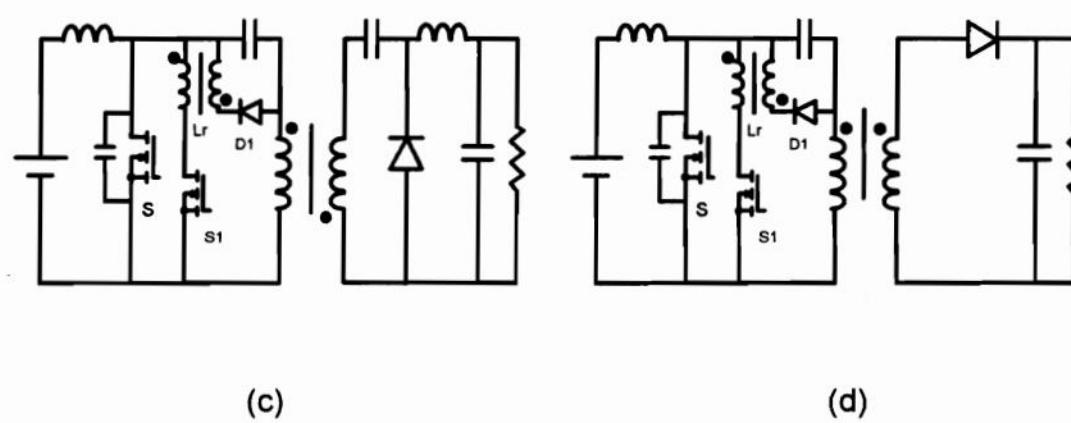
**Fig. 4.13.** Several isolated ZVT-PWM topologies: (a) forward, (b) flyback, (c) Cuk, and (d) SEPIC.
