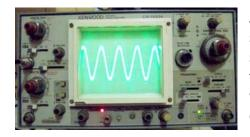
An Oscilloscope is a must for a homebrewer. This single tool can do multi-tasking measurement started from AC or DC voltage, frequency, phase and the most important task is capability to see a signal waveform. By adding a simple external interface, it can be used to see signal at the frequency domain, means a homebrew spectrum analyzer.
