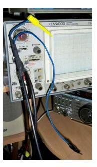
My oscilloscope has input impedance os 1M Ohm 22pf, it is seem to be general for almost oscilloscopes outside there. Knowledge of the oscilloscope's input impedance is quite important to design voltage divider circuit to get a 1X, 10X, 100X or other probes.
