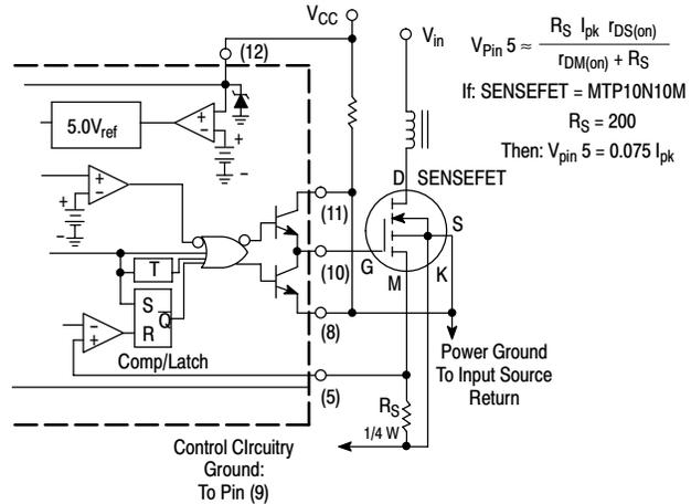
Virtually lossless current sensing can be achieved with the implement of a SENSEFET power switch. For proper operation during over current conditions, a reduction of the  $I_{pk(max)}$  clamp level must be implemented. Refer to Figures 20 and 22.
