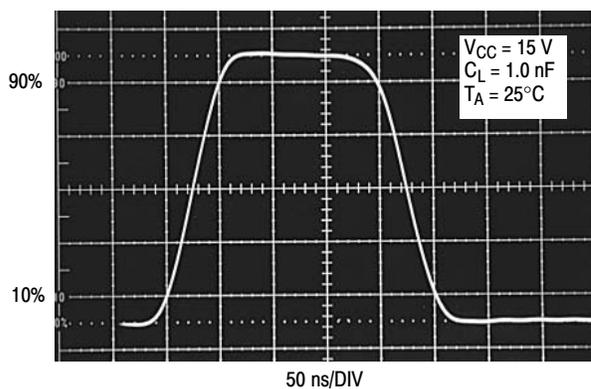
Figure 13. Output Waveform
