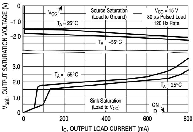
Figure 12. Output Saturation Voltage versus Load Current
