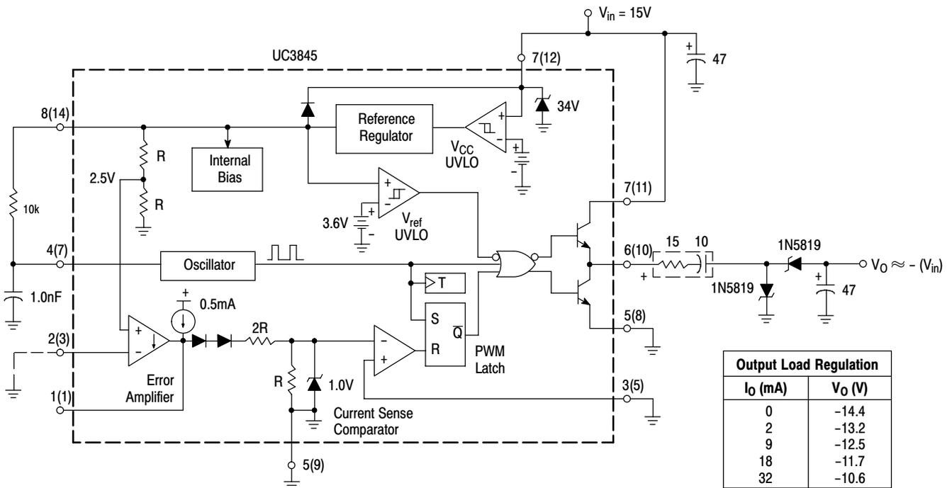
The capacitor's equivalent series resistance must limit the Drive Output current to 1.0 A. An additional series resistor may be required when using tantalum or other low ESR capacitors.
