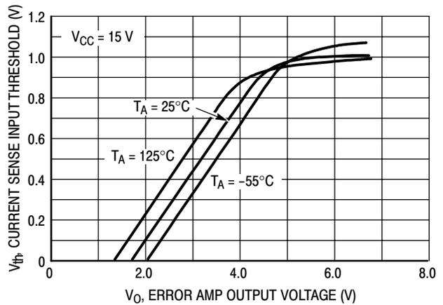
**Figure 7. Current Sense Input Threshold versus Error Amp Output Voltage**
