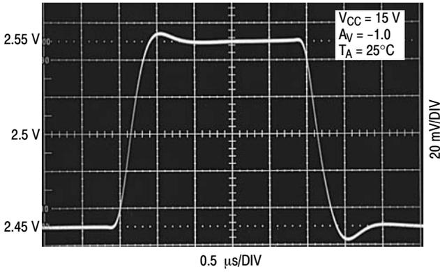
**Figure 4. Error Amp Small Signal Transient Response**
