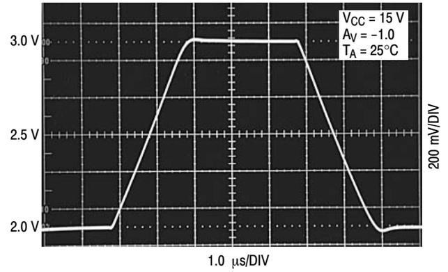
**Figure 5. Error Amp Large Signal Transient Response**
