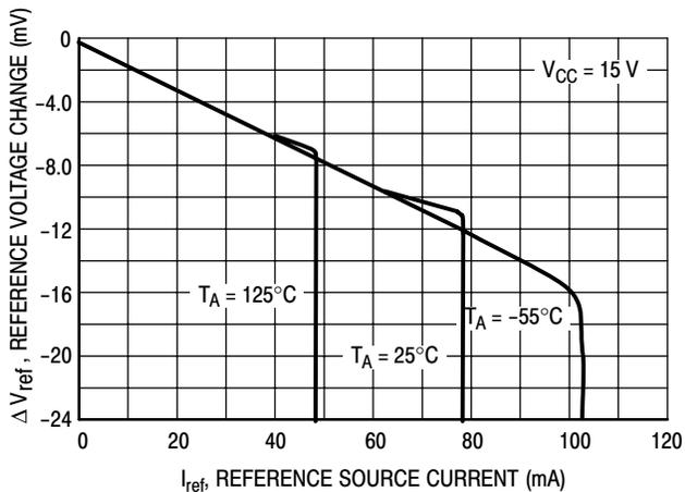
Figure 8. Reference Voltage Change versus Source Current
