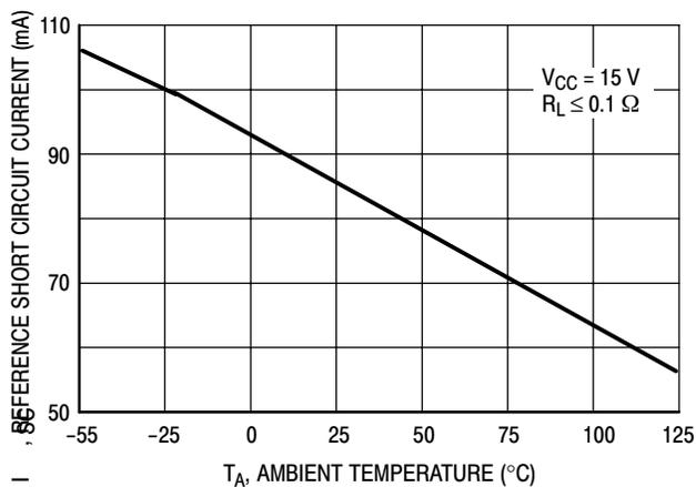
Figure 9. Reference Short Circuit Current versus Temperature
