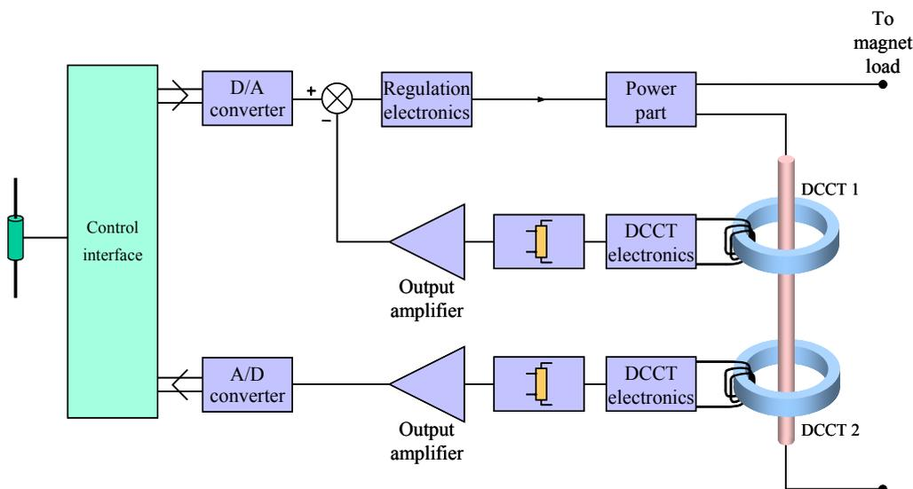
**Fig. 1:** Traditional analog regulation loop
