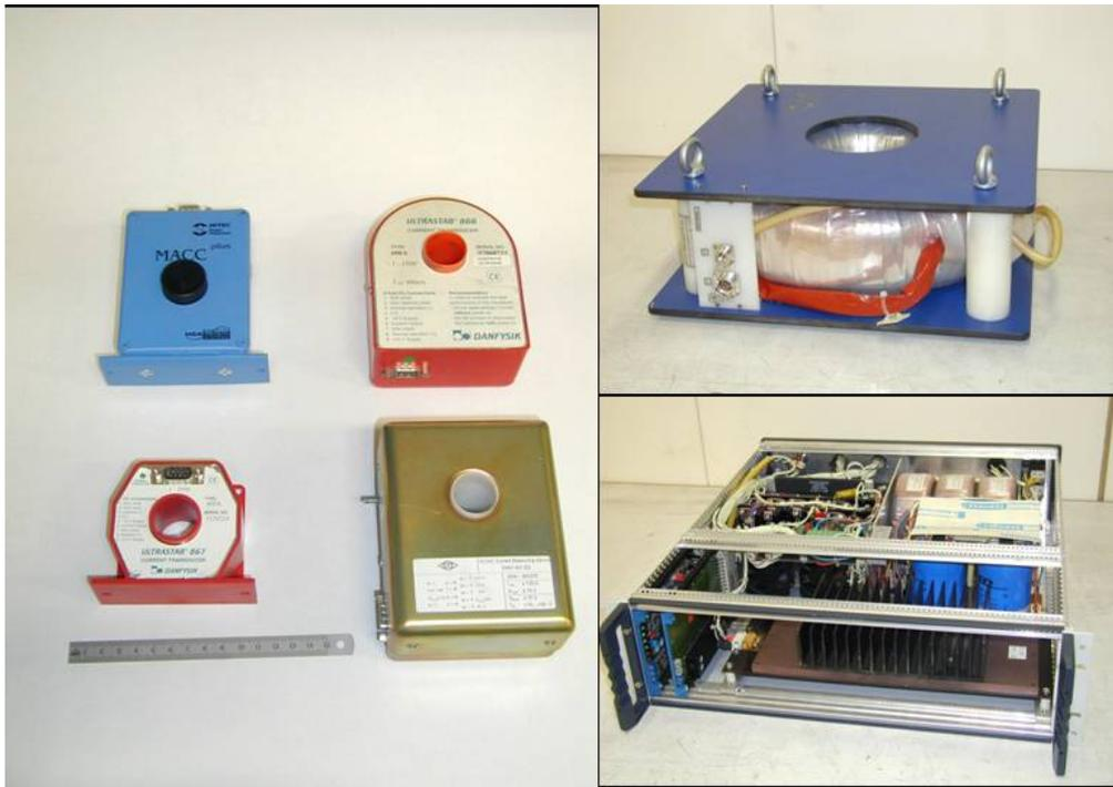
**Fig. 7:** DCCTs of different size and manufacture
