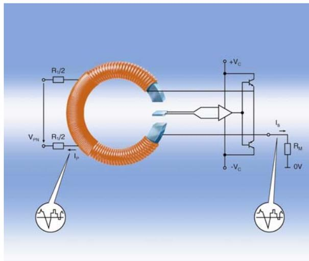
**Fig. 3:** LEM voltage transducer
