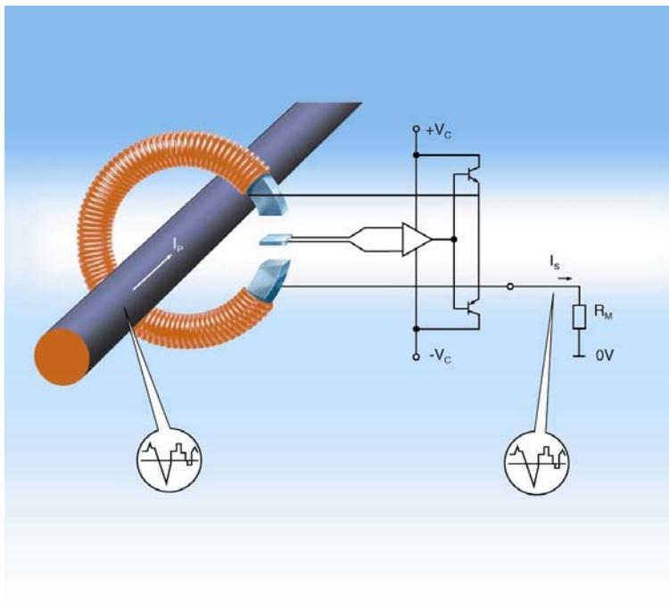
**Fig. 5:** LEM current transducer
