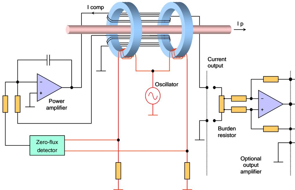
**Fig. 6:** Principle of a zero-flux DCCT
