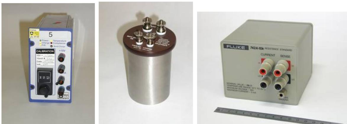
**Fig. 8:** Examples of voltage and resistance standards
