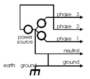
This three phase power system is called THREE-PHASE STAR; FOUR-WIRE; EARTHED NEUTRAL system. This is the most common way used in European wiring systems (and used almost everywhere in Finland), but note that three-phase distribution circuits come in several flavours. There is a distinct difference between those in the US and those in Europe. They are classified as follows:
