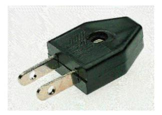
Nowadays, many two-prong devices have one prong wider than the other. This is so that the device could rely (not guaranteed!) on one specific wire being neutral, and the other hot. This is particularly advantageous in light fixtures, where the shell should neutral (safety), or other devices which want to have an approximate ground reference (ie: some radios).
