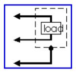
Here the two upper wires are the live and neutral wires. There is not much difference which one of those is live and which one is neutral because modern equipments are designed so that this does not matter. In some countries the power connector is designed so that you always know which wire has live and which has neutral in it. In some countries (for example Finland) the power connector is designed so that it can be put to the connector in two ways.
