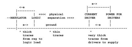
The common mistake is to "daisy chain" the ground by having the ground of the high current item seek it's current path through the ground of the logic. This causes ground spikes on the logic and thus logic errors due to bad voltage levels at the logic chips.
