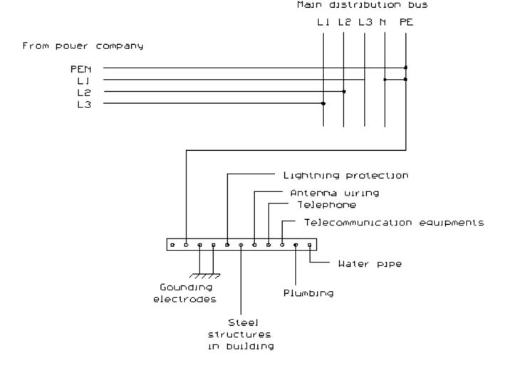
The central grounding bar works as the central point for whole building grounding system and every grounded system in the building is connected to it. The central grounding bar is just a metal bar which connected the grounding wires from the mains power, telephone equipments, antenna wiring, lightning protectors, metal plumbing, water pipes, building steel structures and building grounding electrodes together.
