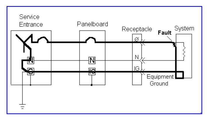
This short circuit situation causes very high current surge to flow in the circuit which will cause the distribution panel fuse to blow almost immediatly. The cureent in short circuit situation can be pretty high because of the low resistance of the mains distribution wiring.
