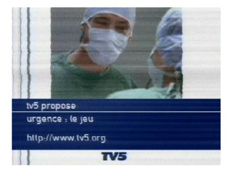
Ad you can see that video signal has strong hummign bars and other interference in it. Those have entered the cable TV signal because of ground loops in the system. Ground loops in the video systems can have following effects:
