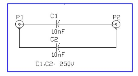
There is one disadvantage of this the circuit breaks the continuous shielding of the antenna cable which makes you antenna cable pick up radio interference more easily (for example radio interference picked by ground loop itself). Usually this is no big problem, but if you notice severe interference then you might have to stop using this isolator. The beast place tu put this isolator (to keep possibility of interference minimun) is just between TV receiver and antenna cable going to wall.
