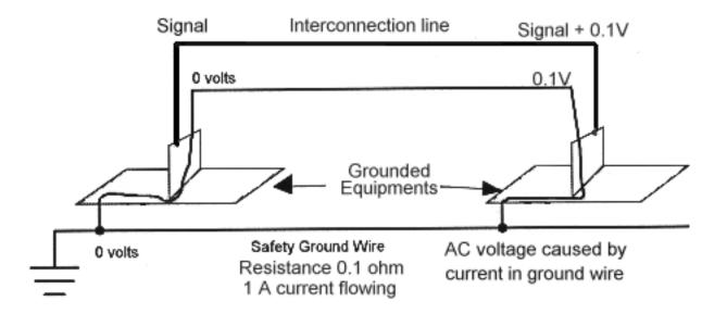
Because there is voltage difference between the ewuipments, the signal in the interconnection wire sees that difference added to signal. This canbe heard as humming noise on the wire because the AC current cause the voltage difference of those ground potentials to be also AC voltage. This is one reason for this 50 Hz or 60 Hz noise you hear in the audio signal (or see in video signal as annoying horizonal bars).
