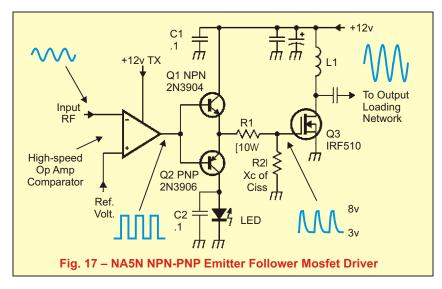
comparator is powered from +12v TX, so that during receive, the output is 0v, disabling the IRF510 drive circuitry.
