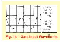
**Figure 14** is an oscilloscope display showing the waveforms one can expect. The gate waveform serves as a great diagnostic tool in evaluating your class D/E/F transmitter.
