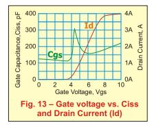
(and other factors) causes a sudden increase in the gate capacitance at Vgs(th). This is illustrated in **Figure 13**, with Vgs(th) at 4.0v. The graph is derived from the data sheets, application notes, and measurements I have made on the IRF510.
