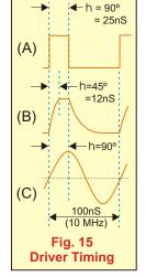
high efficiency of class D/E/F. The 25mA of drive current will save 200mA or more of PA current at 5W QRP. Observing the oscope drive waveform in Fig. 14. note that Ciss charges in 18-20nS at 10.1 MHz This 30M transmitter has an overall efficiency of 82%, which includes the 40mA of key-down current due to the TX mixer, comparator and emitter follower driver providing the date current. This same 18-20nS Ciss charge time will cause a lower efficiency on 20M, as it's approaching
