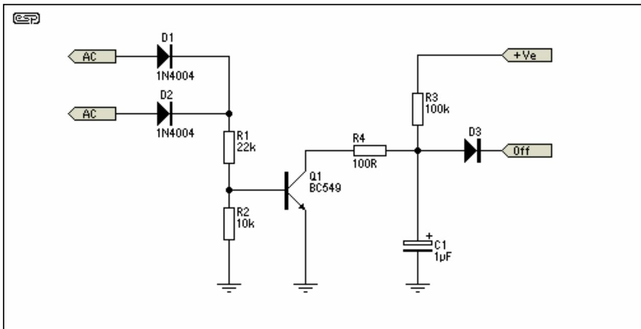
**Figure 3 - Loss of AC Detector**
