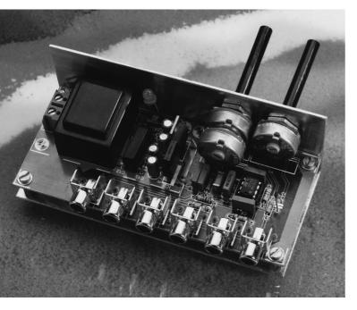
The extension is intended primarily for surround-sound installations that need some boosting of the bass frequencies but where an additional subwoofer cannot be afforded. It is based on a disused mono a.f. amplifier and loudspeaker. If these provide reasonable bass performance, they can be converted into a fairly good subwoofer with the aid of an active low-pass filter—see Figure 1.
