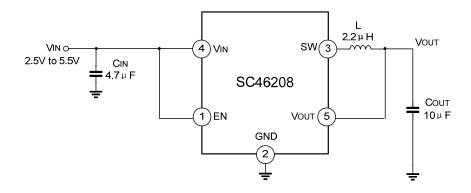
Fig.2: Output voltage fixed regulator
