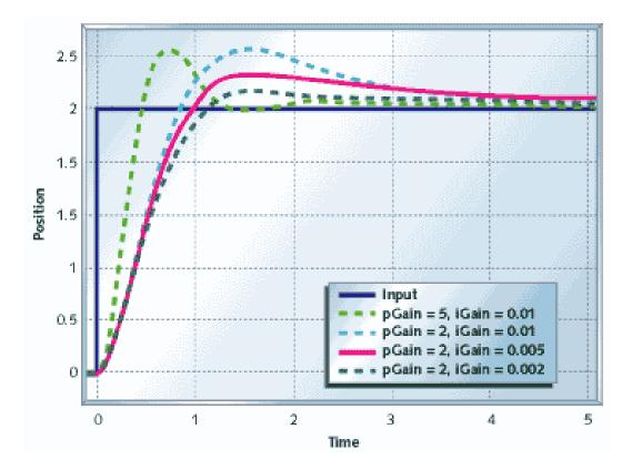
• Figure 13: Motor and gear with PI control
