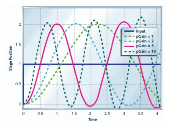
• Figure 9: Precision actuator with proportional feedback vs. time
