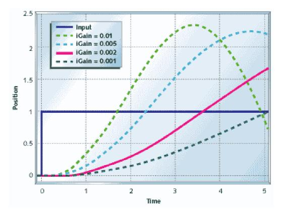
• Figure 11: Motor and gear with pure integral control
