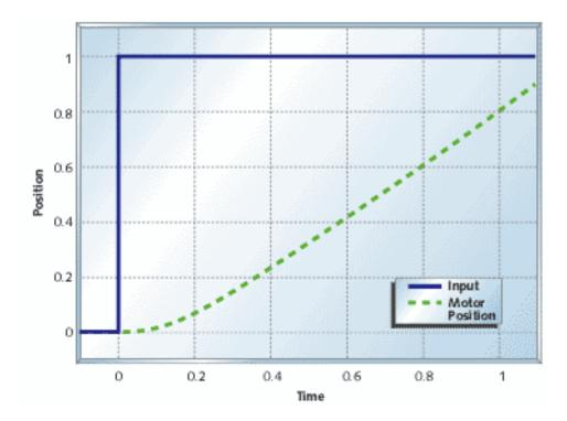
• Figure 3: Motor and gear position vs. time
