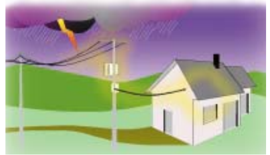
Direct lightning strike on an overhead line
