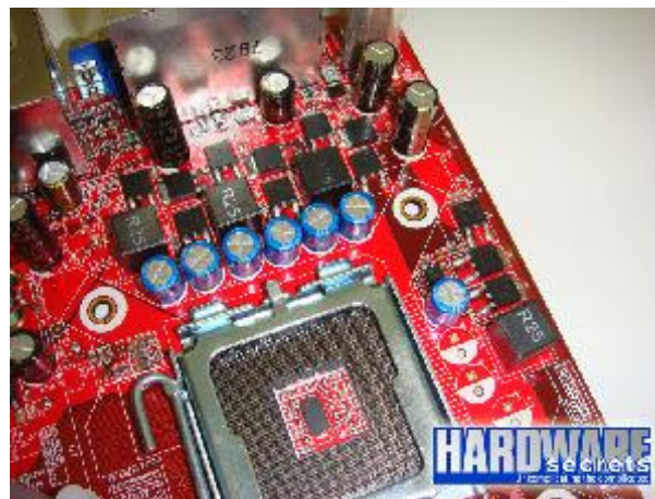
Figure 12: Motherboard with three phases, not four as you could assume.
