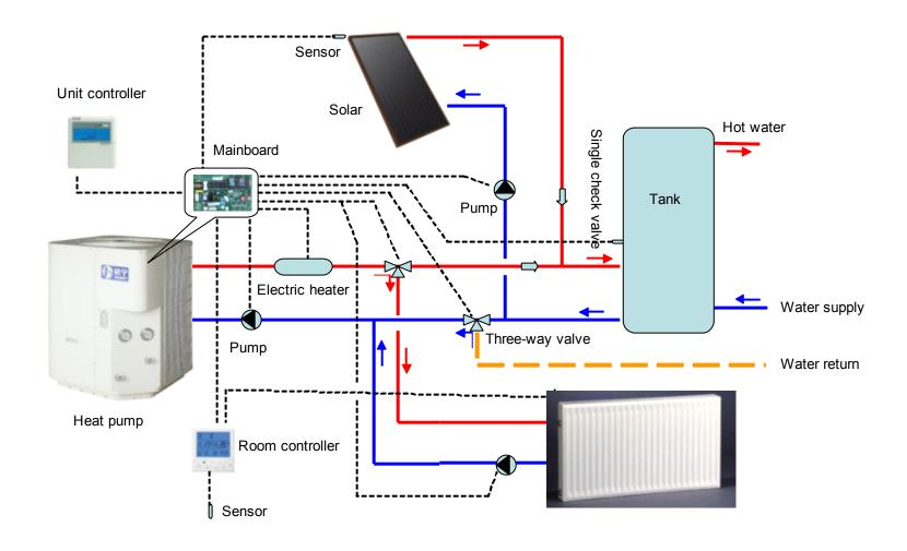
**HOT WATER & HEATING SYSTEM DIAGRAM 2**
