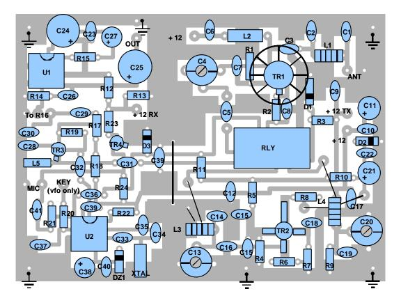
The whole circuit must be put into a metallic box to avoid humming and microphonic effect, common in direct conversion devices, for the same reason the grounding of the PCB must be effective, as shown in the drawing. Note that the TX final stage supply is kept apart from the rest of the circuit, so reducing possible RF feedback and consequent instability, for the same reason the preselector toroids are rotated 90 degrees. The rig may be set up in the following manner :
