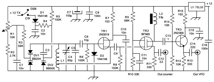
Dealing with a direct conversion circuit, the VFO and the transmitter work on the same frequency, therefore some care must be taken to avoid interference between the two stages. I suggest to put the VFO board into a little tin-plate box (better than aluminium), avoiding to mount it too near the final TX stage.
