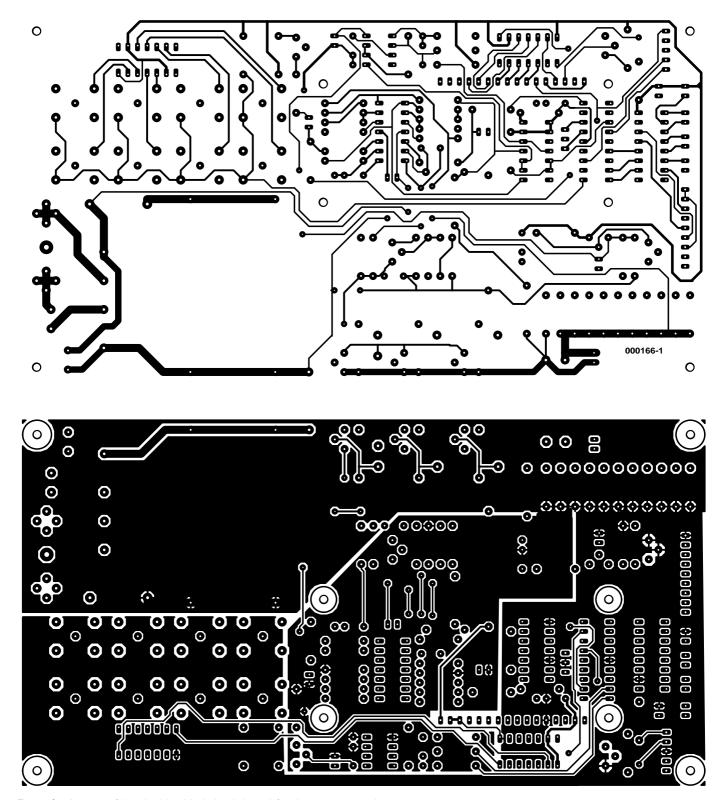
Figure 2a. Layout of the double sided circuit board for the power supply.
