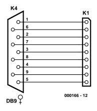
Figure 3. Connections between K1 and the sub-D socket.
