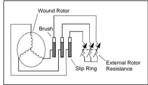
The downside of the slip ring motor is that slip rings and brush assemblies need regular maintenance, which is a cost not applicable to the standard cage motor. If the rotor windings are shorted and a start is attempted (i.e., the motor is converted to a standard induction motor), it will exhibit an extremely high locked rotor current – typically as high as 1400% and a very low locked rotor torque, perhaps as low as 60%. In most applications, this is not an option.
