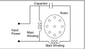
Permanent split-capacitor motors have a wide variety of applications depending on the design. These include fans, blowers with low starting torque needs and intermittent cycling uses, such as adjusting mechanisms, gate operators and garage door openers.
