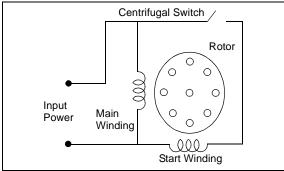
The starting torque is low, typically 100% to 175% of the rated torque. The motor draws high starting current, approximately 700% to 1,000% of the rated current. The maximum generated torque ranges from 250% to 350% of the rated torque (see Figure 9 for torque-speed curve).
