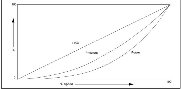
In simple terms, this means that the water flow, head pressure and power are directly proportional to the (speed), (speed)<sup>2</sup> and (speed)<sup>3</sup>, respectively. In terms of mathematical equations, they are represented as:
