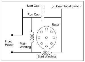
This type of motor can be designed for lower full-load currents and higher efficiency (see Figure 9 for torquespeed curve). This motor is costly due to start and run capacitors and centrifugal switch.
