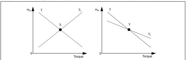
FIGURE 12: TORQUE-SPEED CURVE – SAME MOTOR WITH TWO DIFFERENT LOADS
