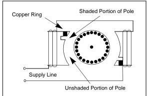
The shaded-pole motor has many positive features but it also has several disadvantages. It's low starting torque is typically 25% to 75% of the rated torque. It is a high slip motor with a running speed 7% to 10% below the synchronous speed. Generally, efficiency of this motor type is very low (below 20%).
