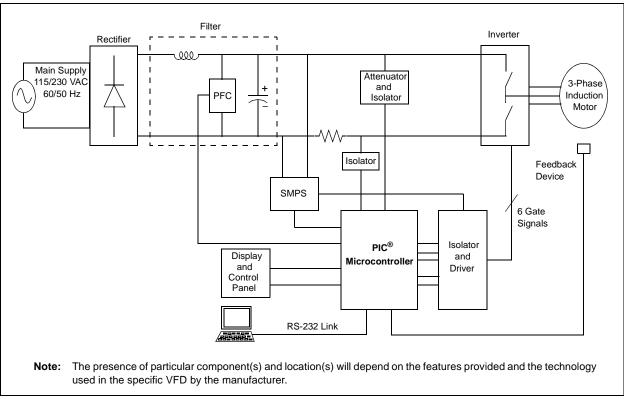
FIGURE 20: TYPICAL VFD
