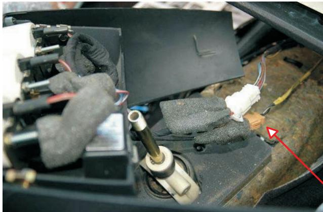
illumination and you'll see the wire running between the 2 sections of the consol. It's a bit fiddly but the plug to the lighter and bulb should come free easily enough and you can now continue to ease the centre consol back and up till its clear.
