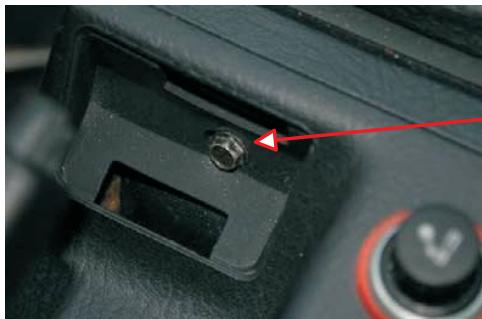
There a little blanking plate in the forward part of the handbrake grab recess that when prised off reveals another black 8mm hex headed bolt to be removed. This secures the centre to the rear/middle consol.
