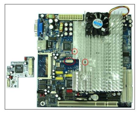
2. Line up the screw-fixing holes of the LVDS-05 module with the screw-fixing holes on the Dual heatsink. The screw-fixing holes and LVDS connector are indicated by red circles above.
