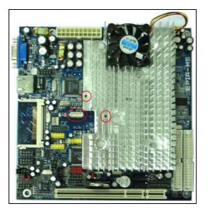
4. Connect the panel power cable, one side onto the LVDS-05 (+12V\_CONN) and the other side onto the PWR FAN connecter on the motherboard.
