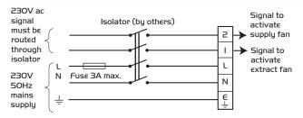
The unit is designed to be wired directly to the mains supply through a fused spur isolator (by others). With the rear section only fixed in position bring the mains wiring through the cable gland in the base of the unit (this gland can be moved to the side position if required.
