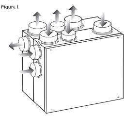
The unit is fitted with two independent fans. Each fan has full speed control for background and boost ventilation rates as well as a run-on timer facility. To recover heat from the extract air an aluminium heat exchanger block is utilised. This heat exchanger can recover over 70% of the normally wasted heat.
