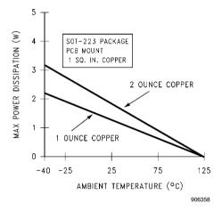
FIGURE 6. Maximum Power Dissipation vs T<sub>AMB</sub> for the SOT-223 Package
