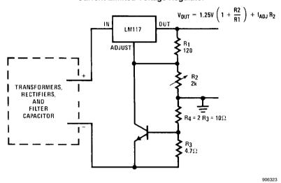
– Short circuit current is approximately  $\frac{600 \text{ mV}}{\text{R3}}$ , or 120 mA
