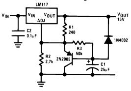
Adjustable Regulator with Improved Ripple Rejection
