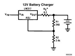
\*R<sub>S</sub>—sets output impedance of charger:  $Z_{OUT} = R_S \left(1 + \frac{R2}{R1}\right)$
