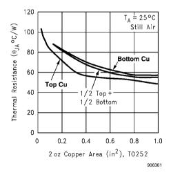
FIGURE 9.  $\theta_{\text{JA}}$  vs 2oz Copper Area for TO-252
