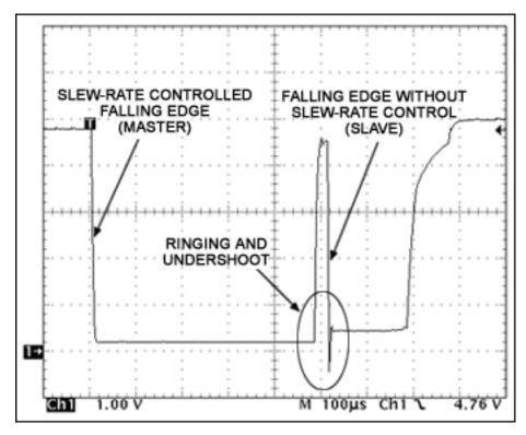
This image shows a bus reset and presence-detect sequence. More importantly, it shows the difference between a slew-rate-controlled edge (master) and an edge without slew-rate control (slave). The falling edge created by the master is clean and does not undershoot or ring. The falling edge created by the slave causes ringing and undershoot on the bus.
