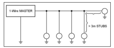
3. Star topology: The 1-Wire bus is split at or near the master end and extends in multiple branches of varying lengths. There are slave devices along, or at the ends of, the branches.
