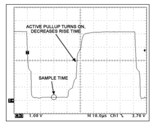
Here is the same active pullup operation in a Read Zero time slot.
