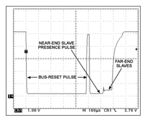
During bus-reset sequences, the active pullup is used to overcome the network weight after the reset pulse, and then again after the end of the presence pulse(s). In this image, the overlap of near- and far-end presence pulses can be observed. The added resistance of the cable between the master and the far-end slave causes the low level to be higher for far-end devices than for near-end devices.
