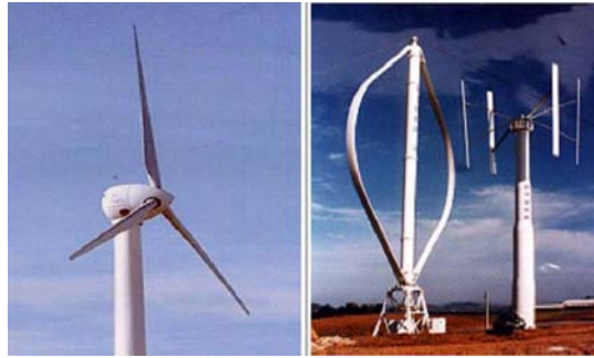
Fig. 2 Classification of wind turbine according to rotating axis type
