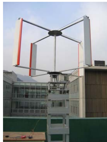
Fig. 4 Cycloidal wind turbine
