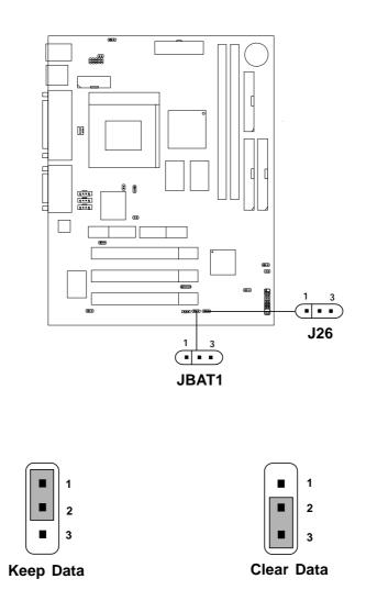
**Note:** You can clear CMOS by shorting 2-3 pin, while the system is off. Then, return to 1-2 pin position. Avoid clearing the CMOS while the system is on, it will damage the mainboard. Always unplug the power cord from the wall socket.
