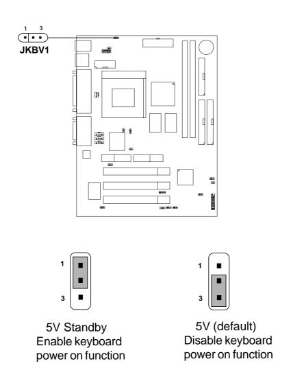
**Note:** To be able to use this function, you need a power supply that provide enough power for this feature. (750mA power supply with 5V Stand-by)
