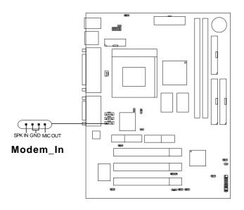
SPK\_IN is connected to the Modem Speaker Out connector. MIC\_OUT is connected to the Modem Microphone In connector.
