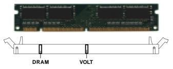
3. The plastic clip at the side of the DIMM slot will automatically close.
