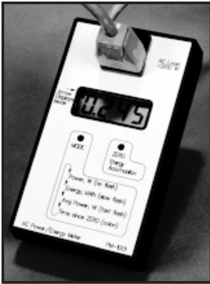
Photo 1—Here's my dream come true—a hand-held portable AC power meter.
