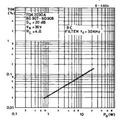
The diagram of Figure 26 originated by SGS-THOMSON can be used to find the Slew-Rate (SR) required for a given output power or voltage and a TIM design target.
