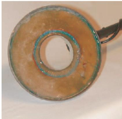
**Fig 11:** Coils glued in
