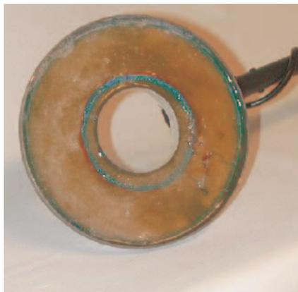
**Fig 11:** Coils glued in
