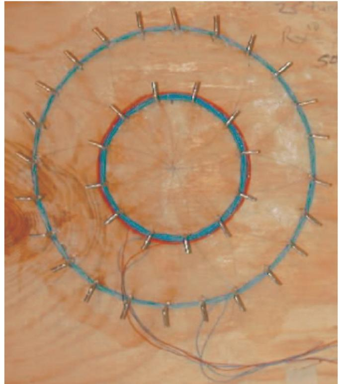
Fig 1: Plywood base with L-hooks screwed in
