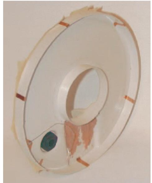
**Fig 6:** Copper strips from the side
